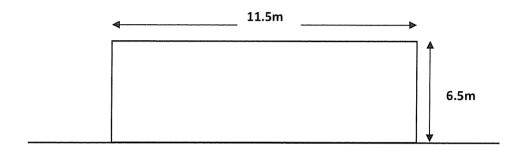
Note that these dimensions include a clearance envelope that permits the safe passage of a load with sufficient tolerance to clear any obstructions.
