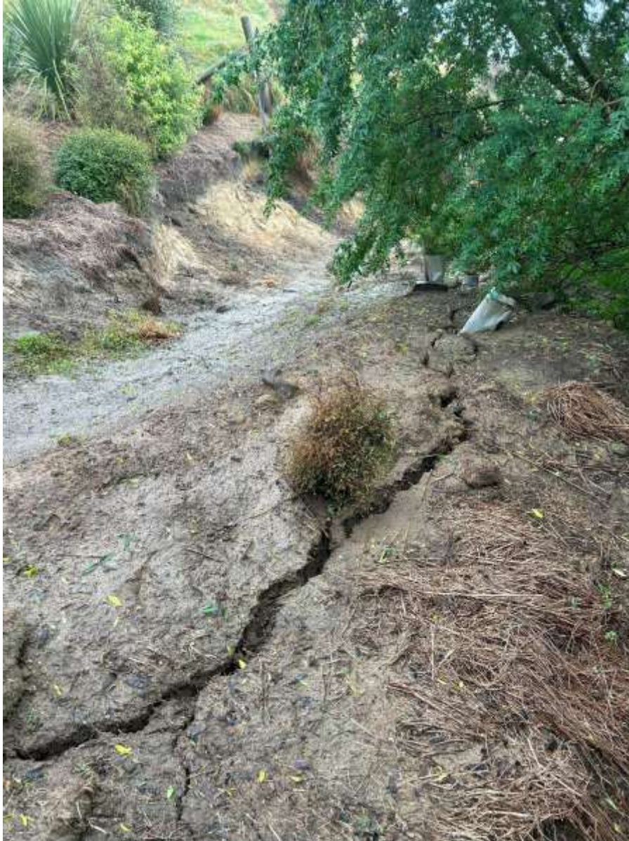
Photo 7. Tension Cracks within Zone D2.
