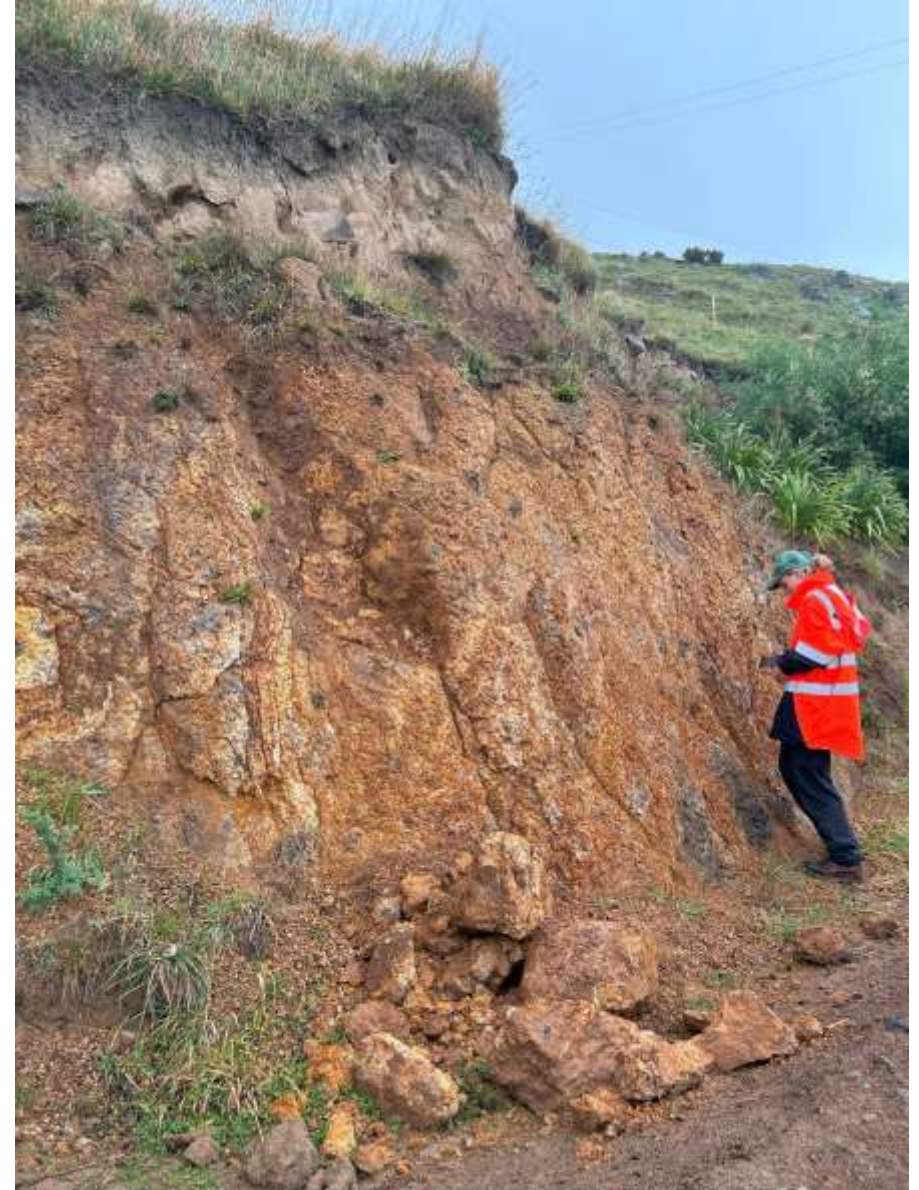
Photo 8. Volcanic Tuff material with open defects (Dip/Dip Direction Measured).
