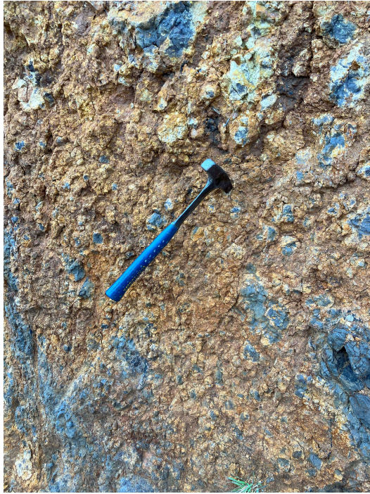
Figure 1 Highly weathered pyroclastic layer visible in the road cut. Basalt clasts are visible in the deposit, presenting as the obvious grey areas, within the browner matrix material
