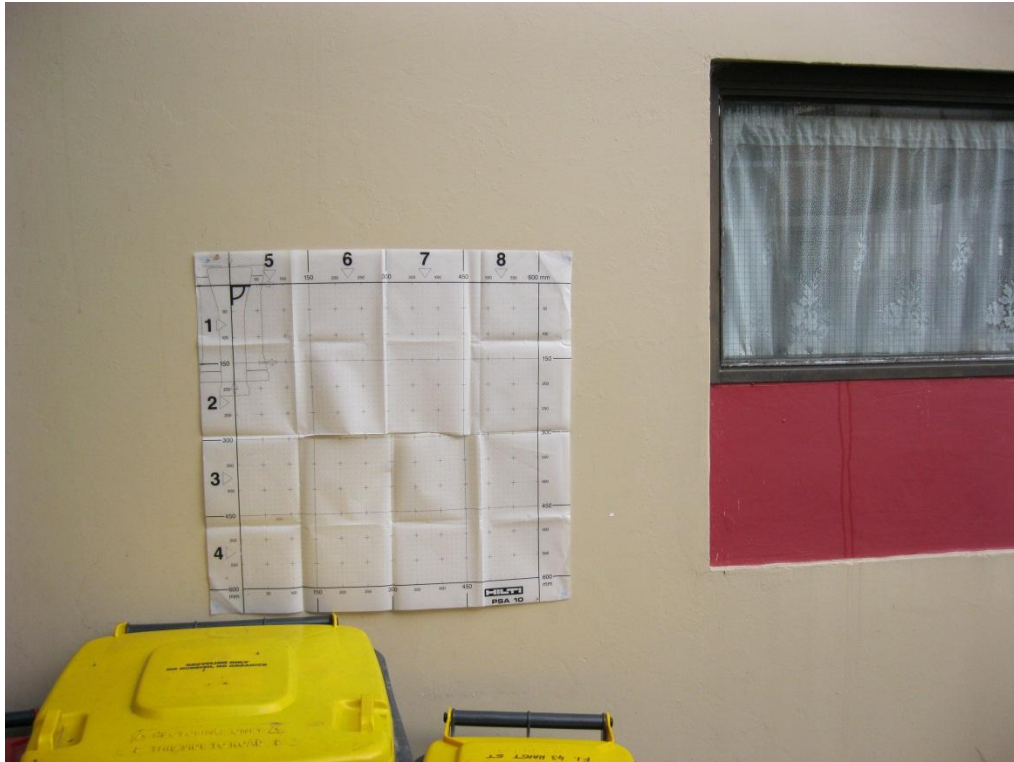
Photograph 5 location of Hilti Ferroskan of wall at ground floor.
