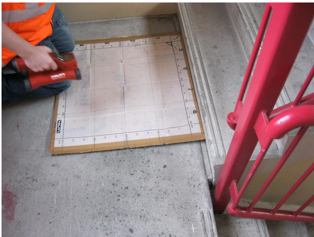
Photograph 5 location of Hilti Ferroskan of wall at ground floor.
