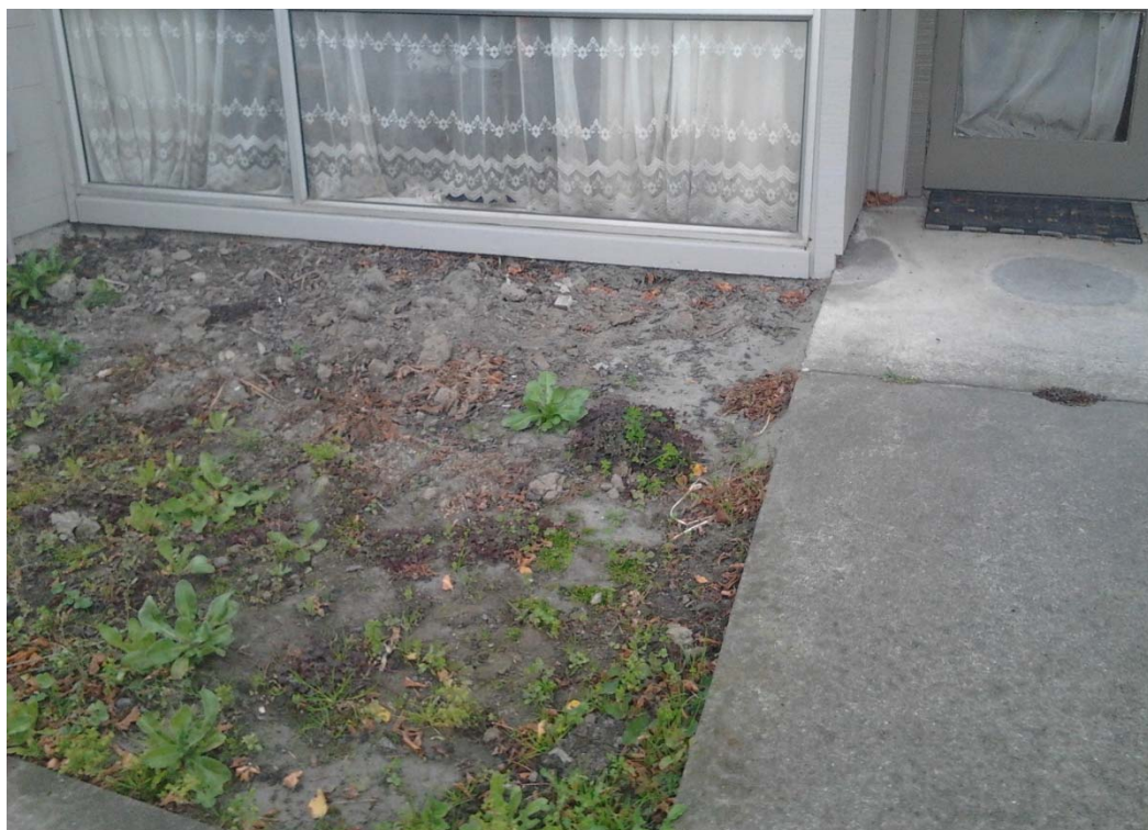
■ Figure 10 Remaining evidence of liquefied material ejecta
