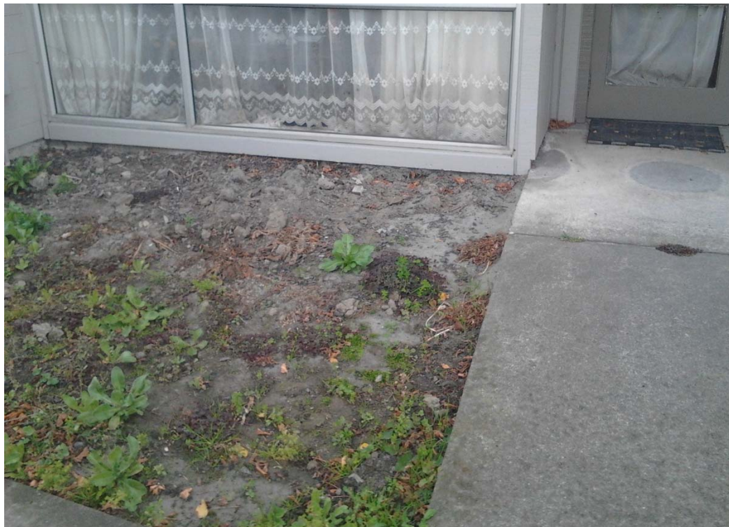
■ Figure 10 Remaining evidence of liquefied material ejecta
