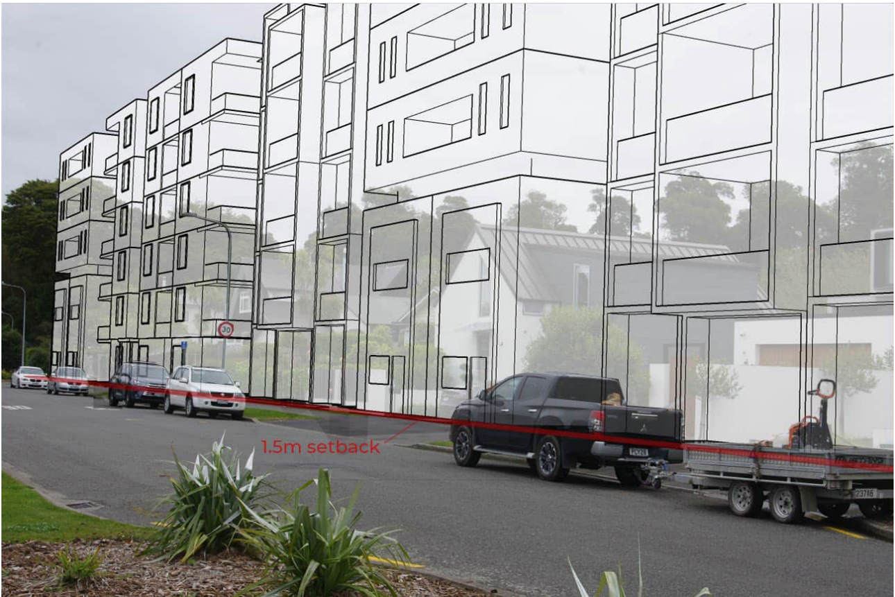
Figure 22: Rata Street looking northwest towards Pūtaringamotu Riccarton Bush, with graphic overlay showing 20m height limit and possible apartment configuration under the NPS-UD Built Form Standards . Outcome may vary through High Density Residential Standard provisions.
