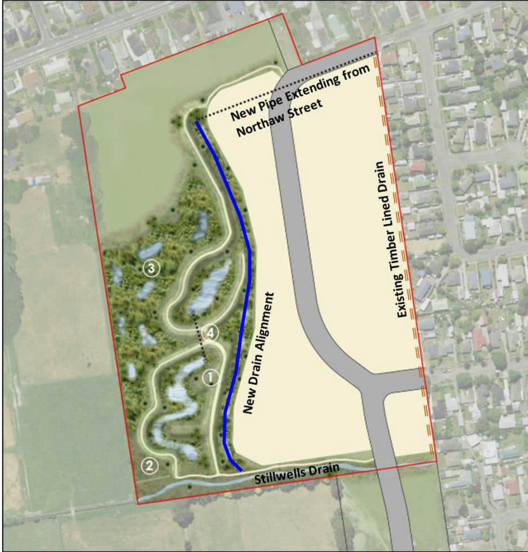
Figure 10. Realignment of Timer Lined Drain
