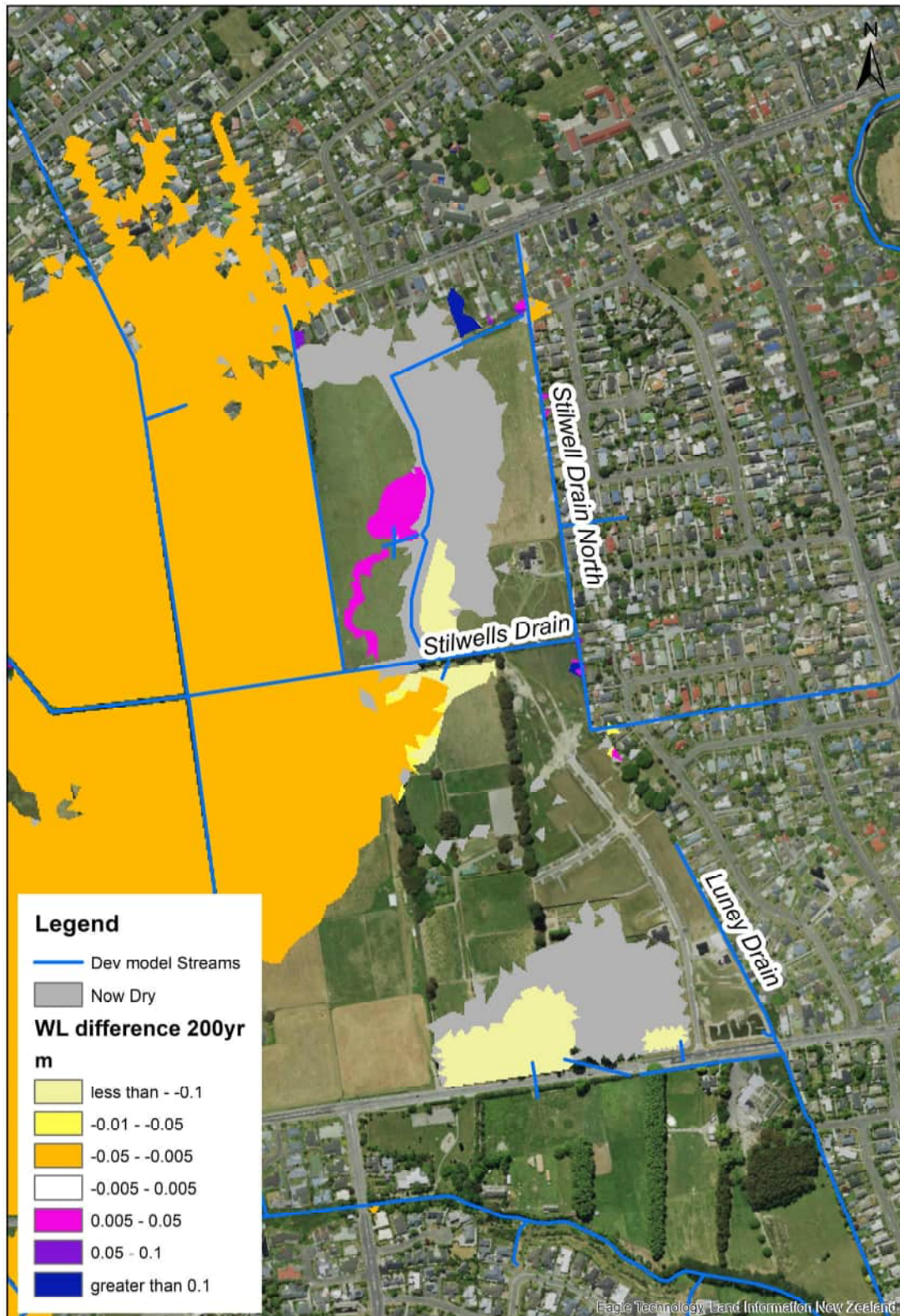
Figure 6: Development - Base, Max Water Level Difference
