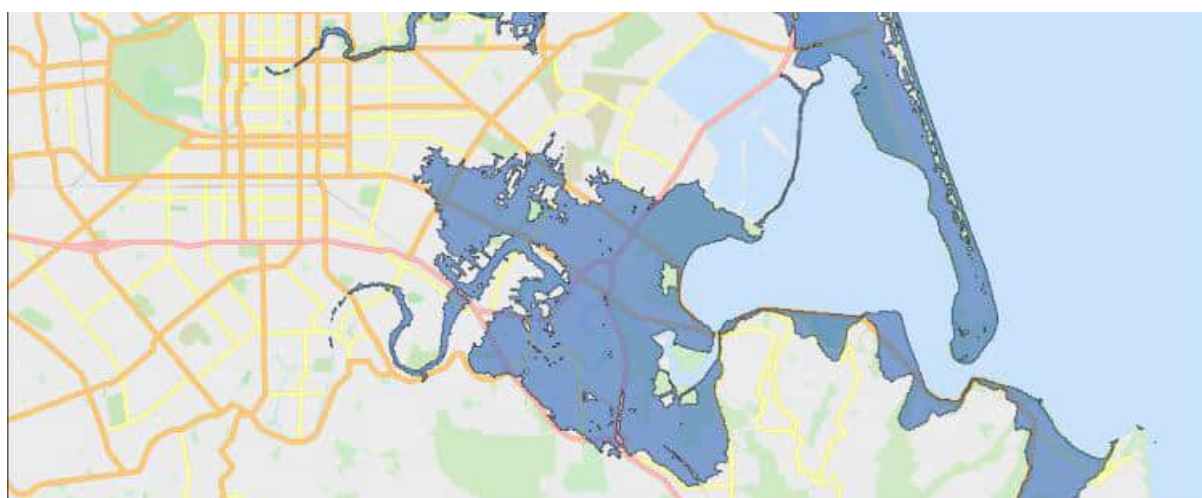
Figure 2: Full extent of 1:500-year tsunami hazard with 1.06-metre sea-level rise applied.
