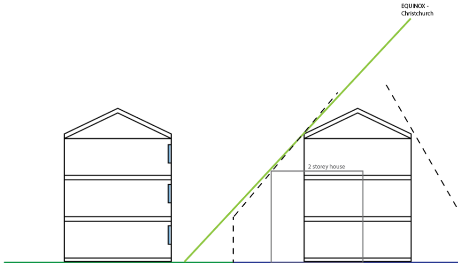
Figure 4: Using a 3m and 50 degree recession plane, the shading from a two- and three-storey house is similar at the equinox.
