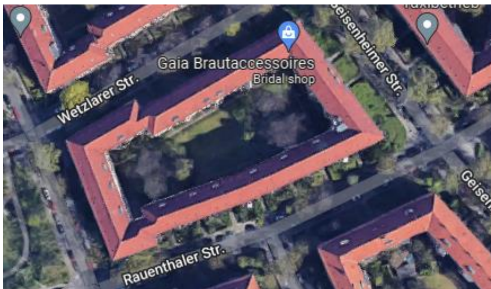
Figure 415: A 6 storey perimeter block in Berlin, Germany with a site coverage of approx. 33% across the entire block. (Source: Google Maps)
