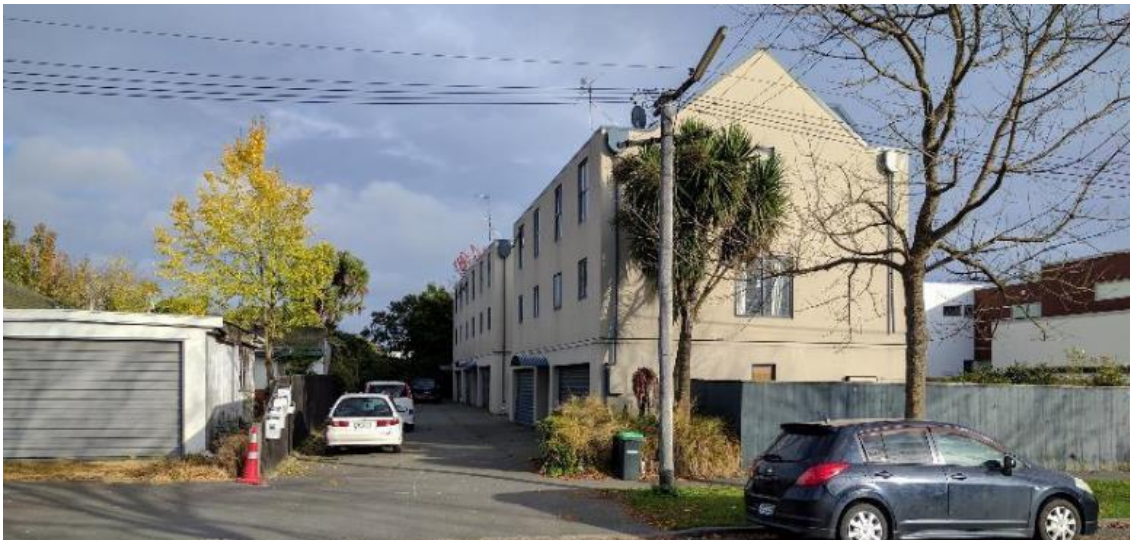
Figure 25: No ground floor living with garaging dominating the ground floor reduces any opportunity for passive surveillance over the journey between the street to the front door.
