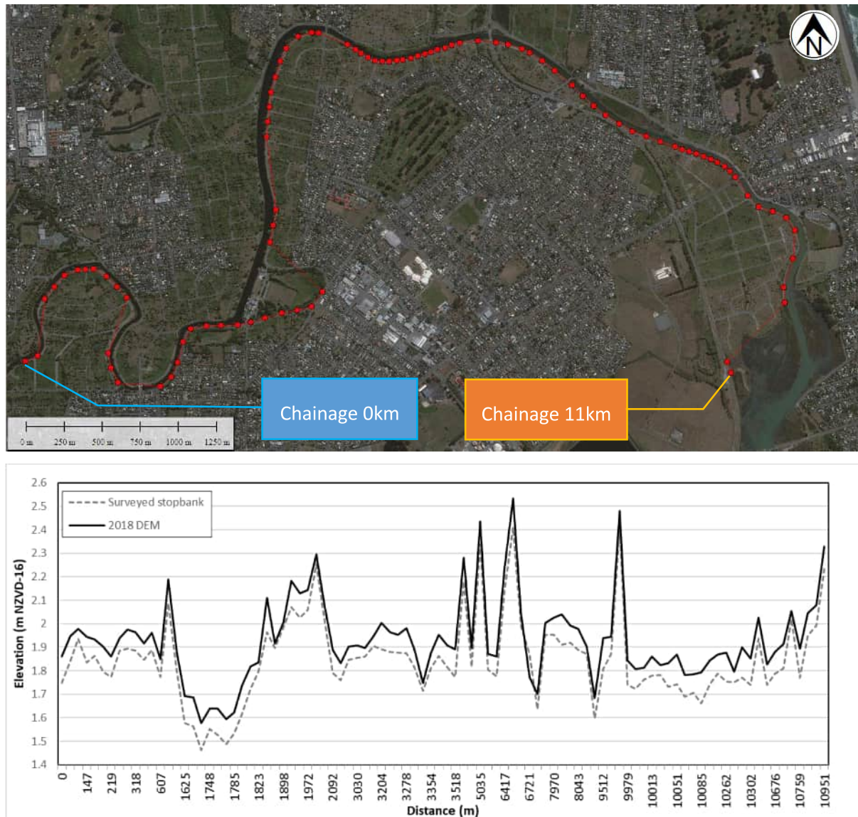
Figure 6.5: Right stopbank map (top panel) and difference between stopbank elevations in 2018-2019 DEM and surveyed levels along the right bank of the Avon River (lower panel).
