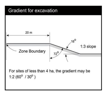
(d) No excavation shall cut below a surface with a gradient of 3 (horizontal) to 1 (vertical) measured from a point commencing 10 metres from the toe of any existing or consented stopbank (see diagram below).
