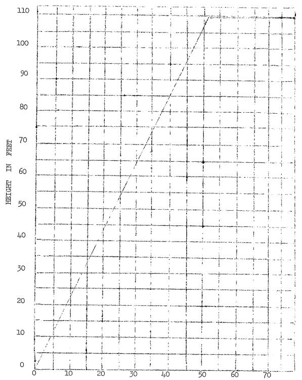
(Note: This graph illustrates only the case where an angle of 65 degrees is adopted. With any other angle an appropriate graph should be prepared, and the reference to the angle in clause 3(3)(b) of ordinance V, amended accordingly. Whatever angle is used should be inserted under the heading "Height-control Line" in the tables of bulk and location requirements for commercial and industrial zones.)
