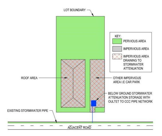
Net stormwater attenuation volumes for below-ground attenuation devices are presented below in Table 1.
