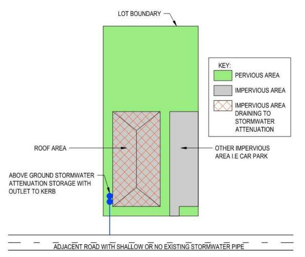
Net stormwater attenuation volumes for above-ground attenuation devices are presented below in Table 2.
