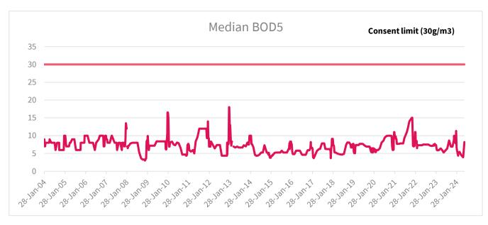
The median concentration of five-day biological oxygen demand in the treated wastewater has not exceeded the consent limit of 30 grams per cubic metre since records were kept starting in 2004.
