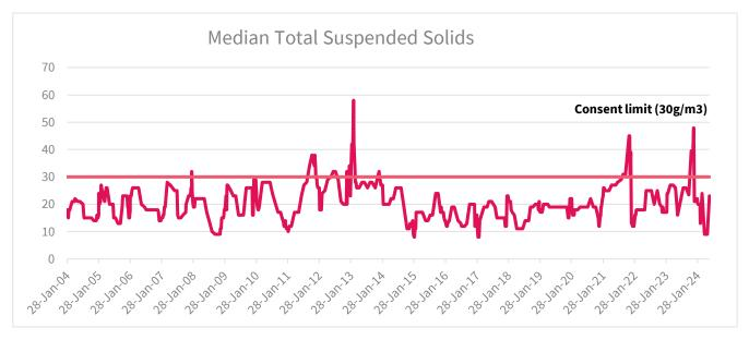
The median concentration of suspended solids in the treated wastewater has not often exceeded the consent limit of 30 grams per cubic metre since records were kept starting in 2004.
