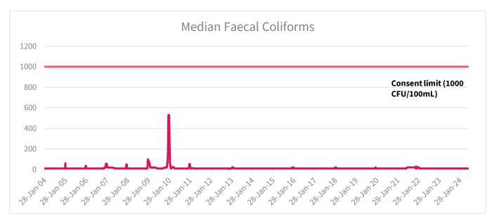
The median concentration of five-day biological oxygen demand in the treated wastewater has not exceeded the consent limit of 1,000 coliform forming units (CFU) per 100 millilitres of treated wastewater since records were kept starting in 2004.
