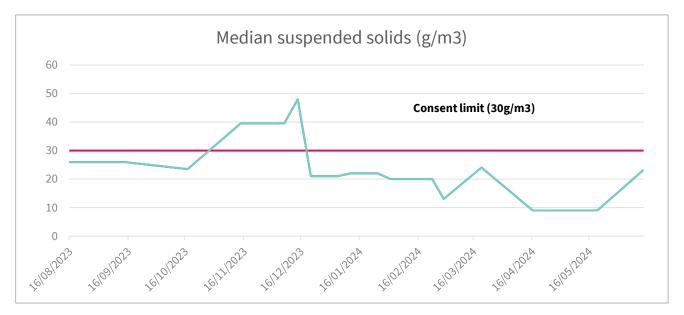
There have been three exceedances of the TSS consent Limit sampled over the year, with 39.5g/m3 on 14/11/20243 and 7/12/2023 and 48g/m3 14/12/2024. These exceedances occurred during the busy summer period where the flow through the plant is at such a high volume that the normal settling time is not achieved.
