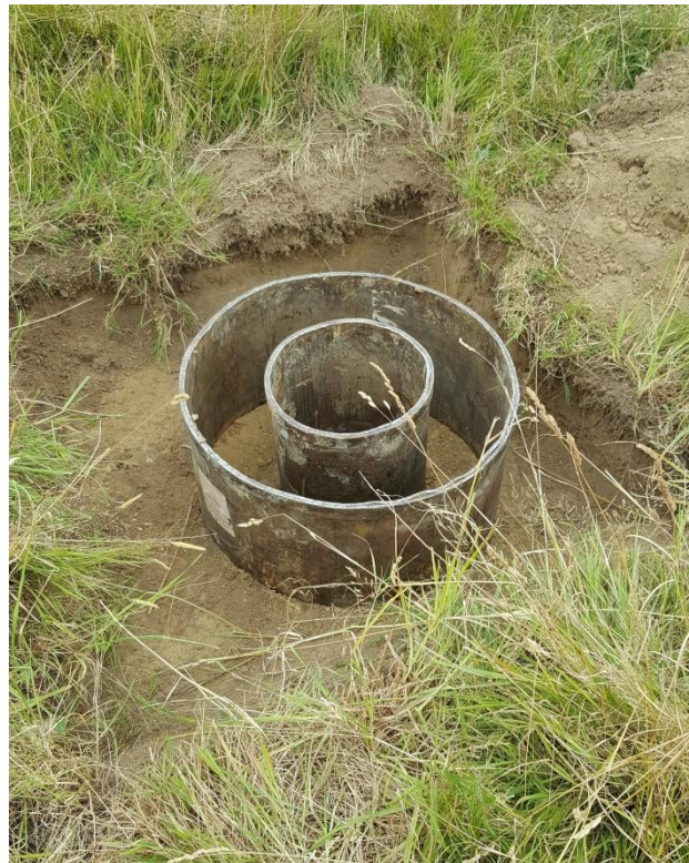
Photograph 5: Infiltration Test IT107 sub-surface infiltration test within Robinsons Bay (Site 107).
