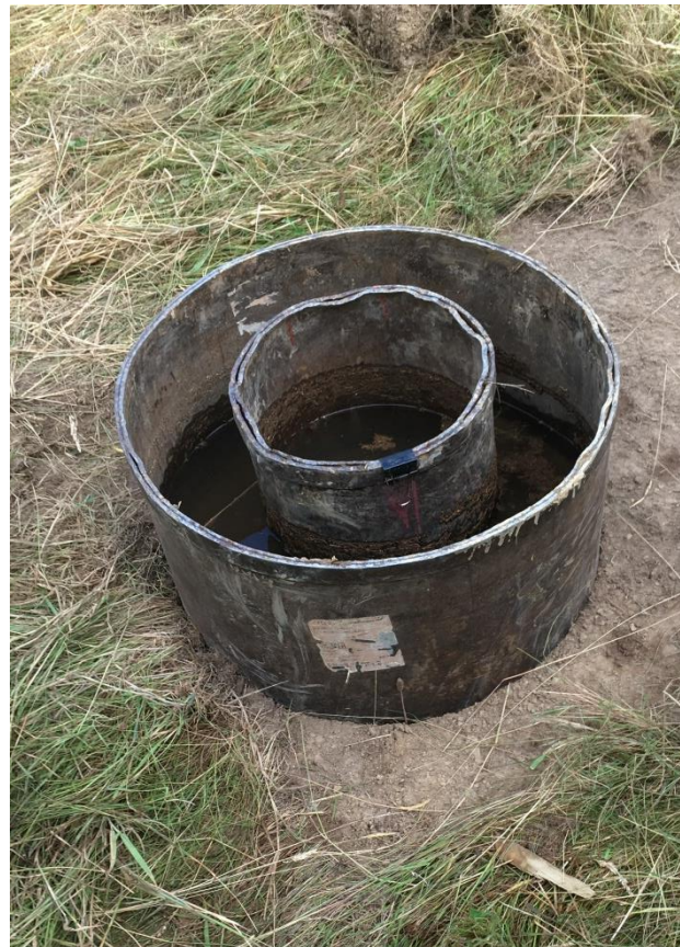
Photograph 2: Infiltration Test IT101 surface infiltration test within Robinsons Bay (Site 101).
