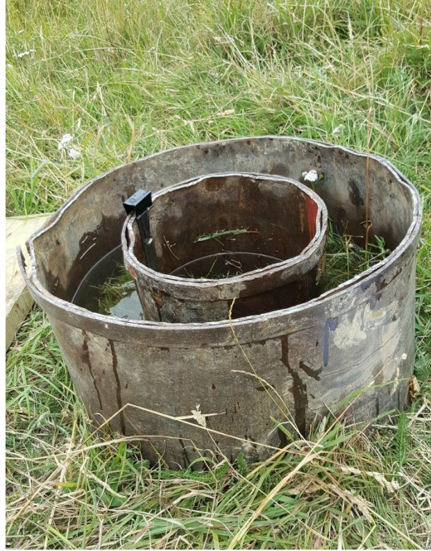
Photograph 4: Infiltration Test IT107 surface infiltration test within Robinsons Bay (Site 107).
