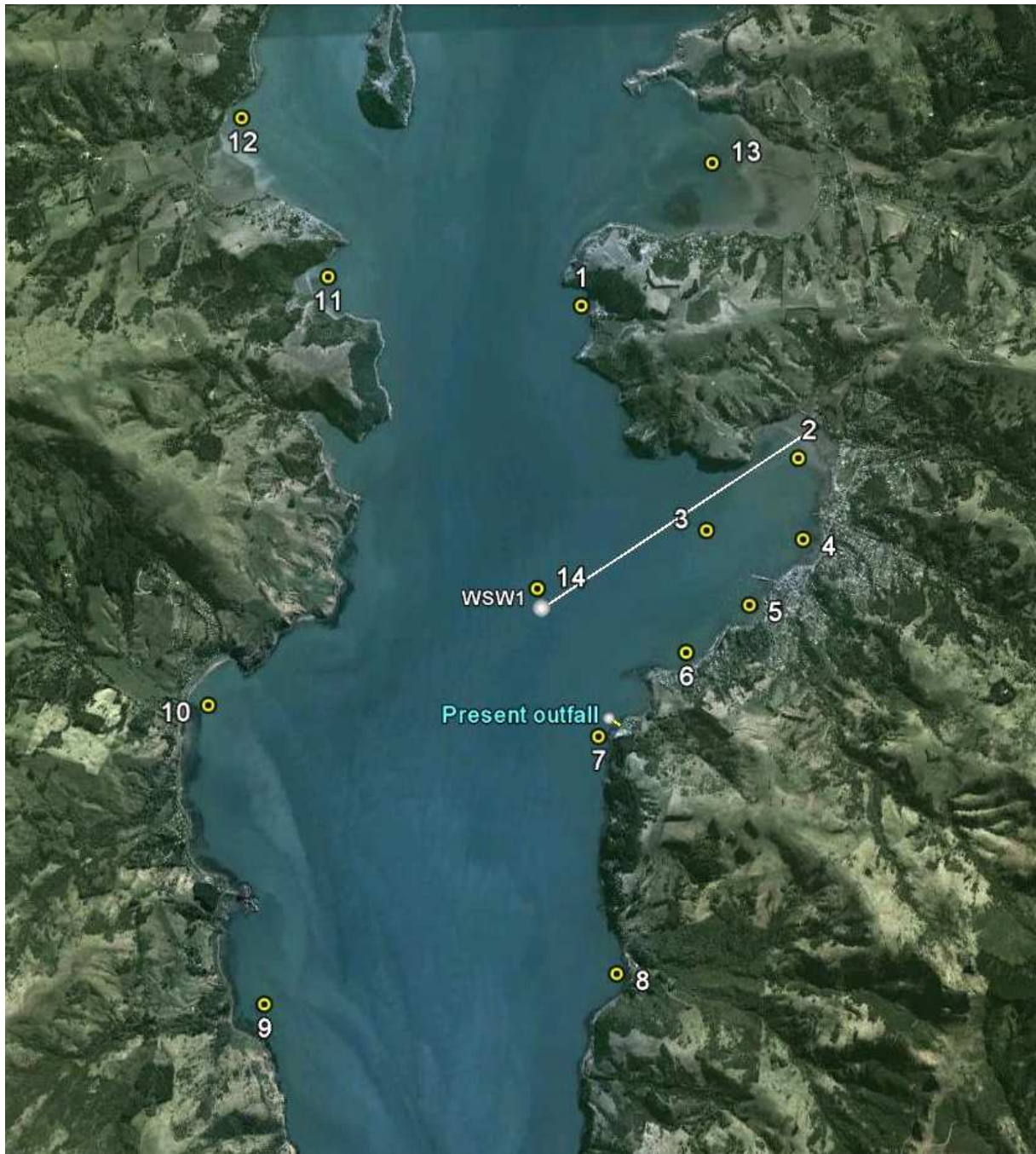
Figure 5-2: Specified sites for which total dilution plus inactivation and concentration-reduction factors were determined. White line is proposed 2.5 km outfall alignment and yellow line near site 7 is the existing outfall.
