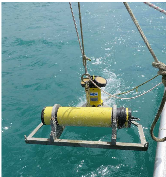
Figure 4-2: Sea-bed mooring frame comprising the 500 kHz SonTek ADP and acoustic mooring release being lowered from the NIWA vessel.
