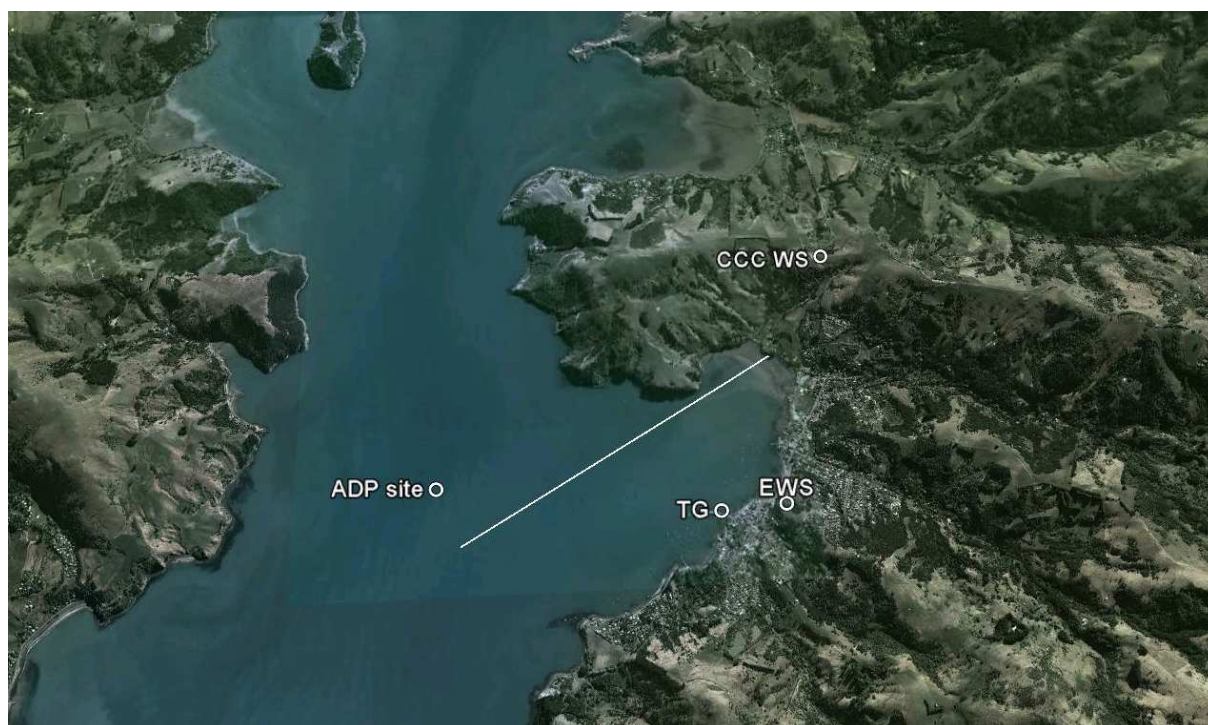
Figure 2-1: Location of wind, tide-gauge and ADP current-meter stations in Akaroa Harbour. [Background image: DigitalGlobe, Google Earth].
