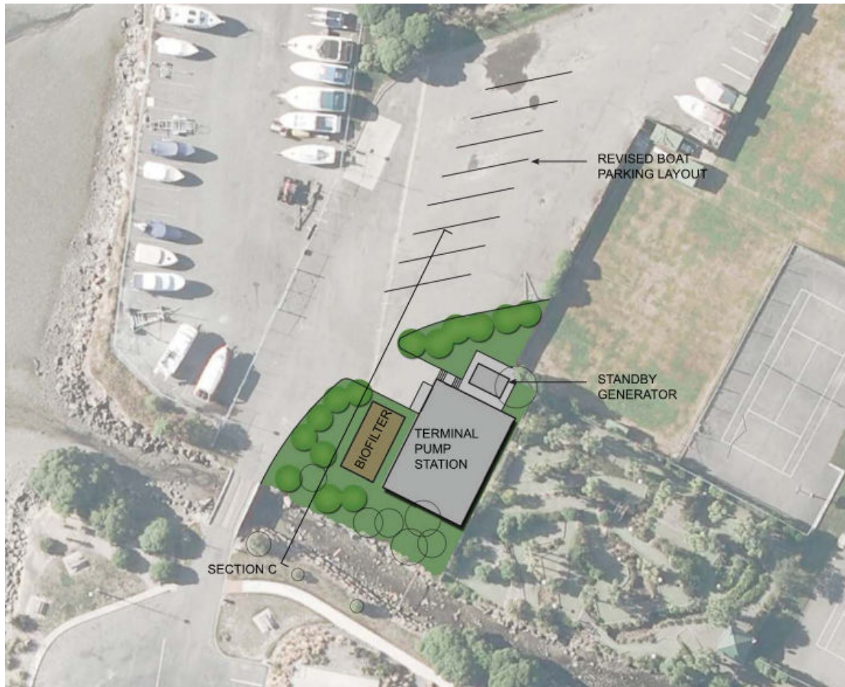
Figure 4-3 Layout of Terminal Pump Station
