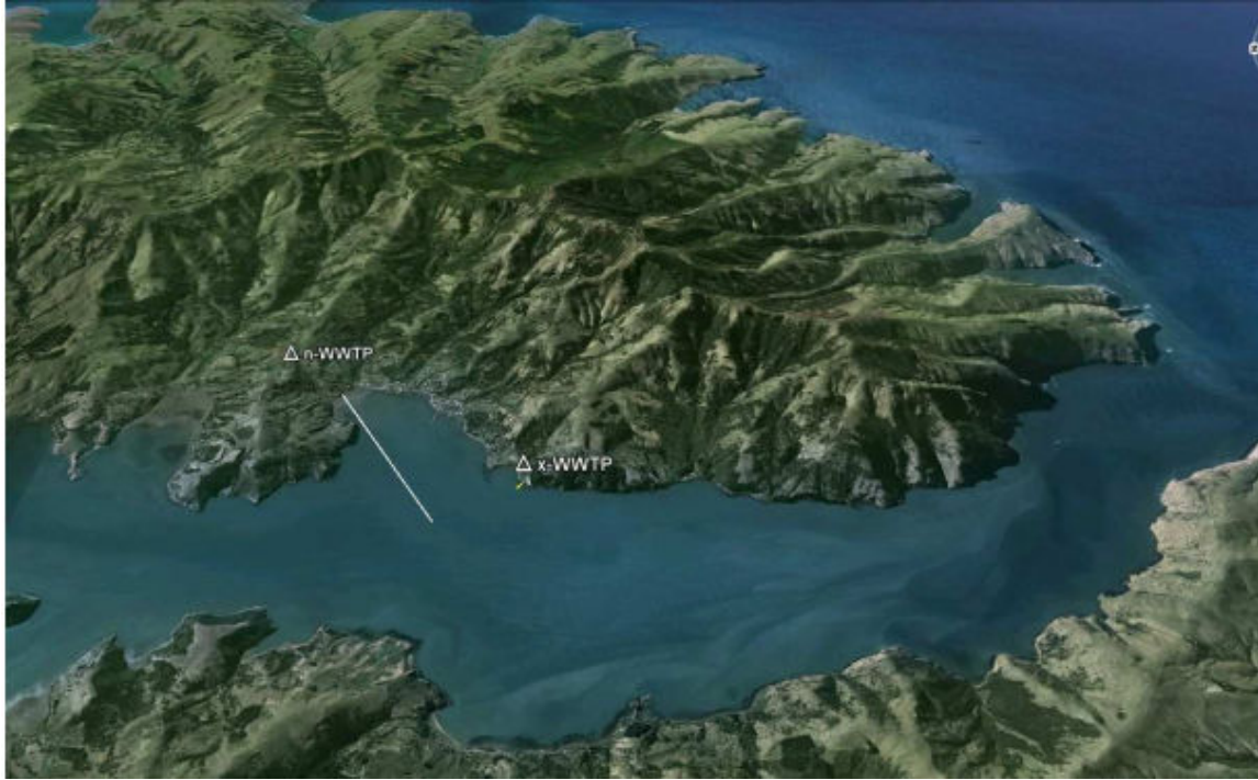
Figure 4-9 Akaroa Harbour and location of existing treatment plant (x-WWTP) and short 100m outfall (yellow) and proposed treatment plant (n-WWTP) and 2.5km outfall (white) Akaroa Harbour
