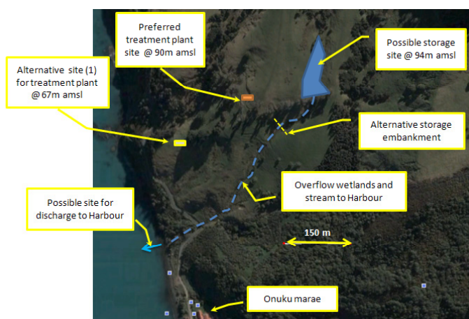
Figure 5.4: Akaroa South Storage Reservoir, Treatment Plant and Irrigation Area Location Options (ecoEng, Jan 2010)
