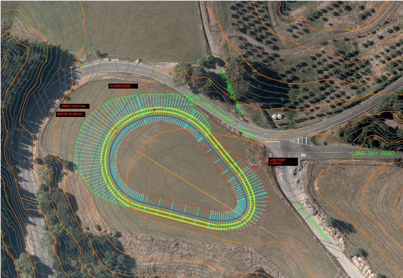
Figure 5-1: Geometric Design of Possible Storage Pond Opposite WWTP (Site 10)
