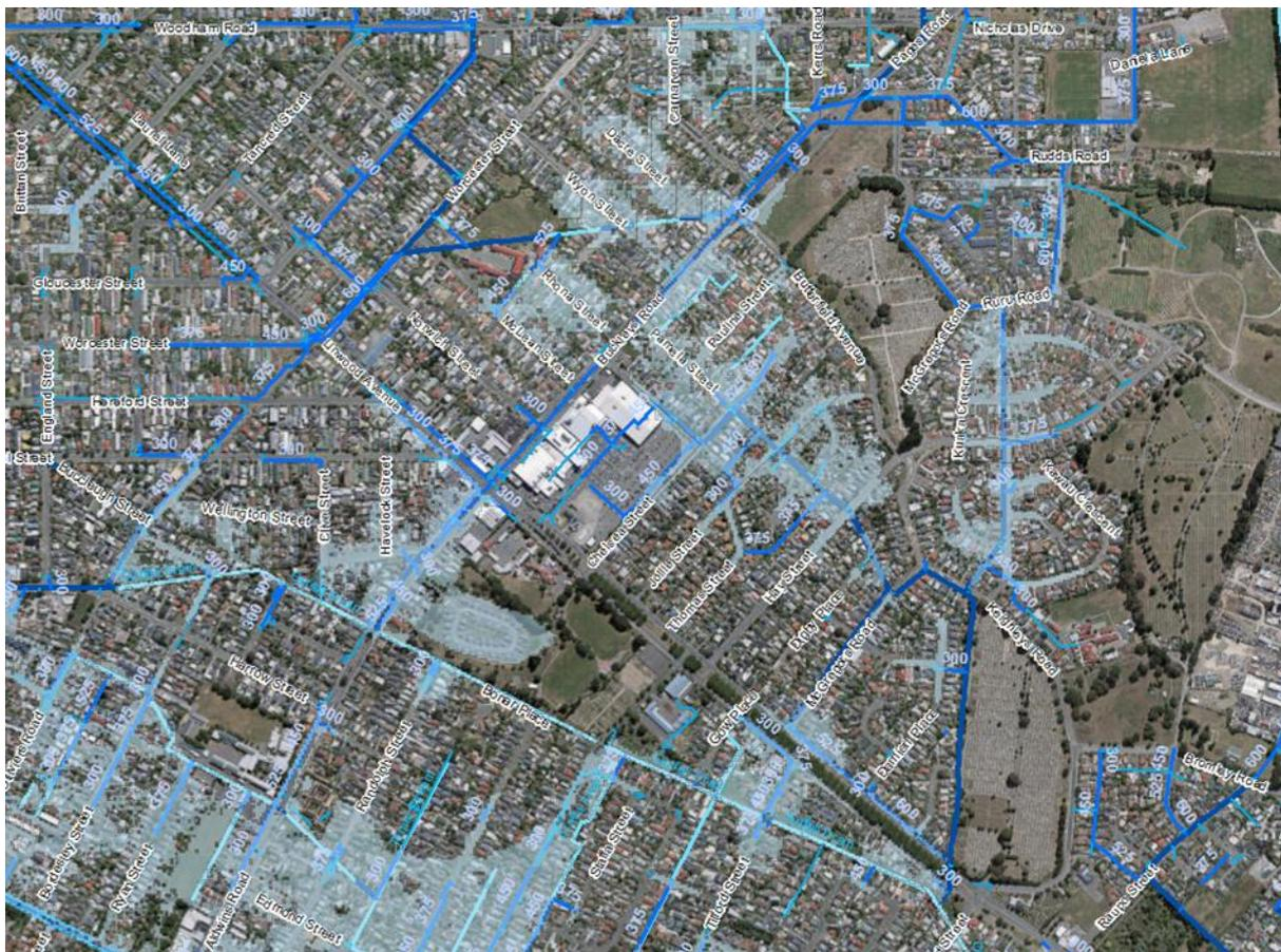
Figure 13: 50 year average recurrence interval flooding event – from model results.
