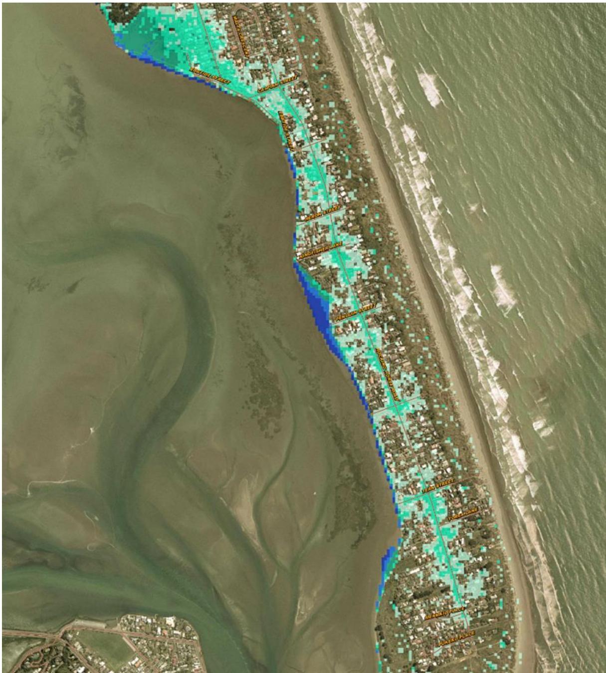
Figure 14: 50 year average recurrence interval flooding – (‘Rain-on-grid’ model, 11.1 m tide)
