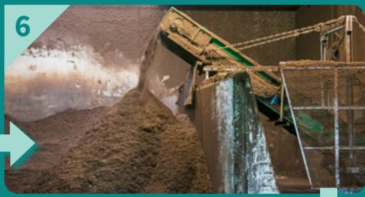
The compost is screened – this separates the finer compost from sticks and other large material, which are known as tailings. The finer compost is then stored onsite for a maximum of 48 hours before being removed.
