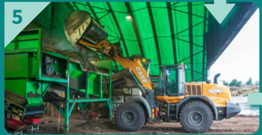
Loaders move the compost from the enclosed tunnels to a covered outdoor area for screening. This photo shows the compost being lifted into the screening area.
