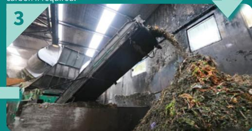
Material goes through a shredder to break it down. A probiotic is added to accelerate the composting process.
