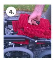
Pull upwards on the carry handle to complete the collapse.
