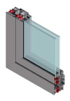
A small plastic barrier, as shown in red, reduces heat loss and condensation.
