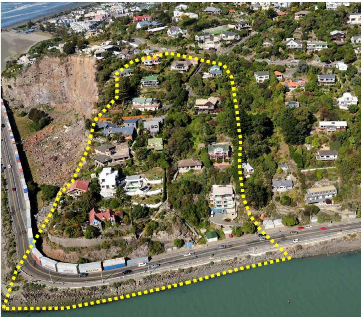
**Figure 3** Aerial view of the Deans Head mass movement is within the yellow dashed lines (approximate extent only – refer to Figure 2 for the mapped extent).
