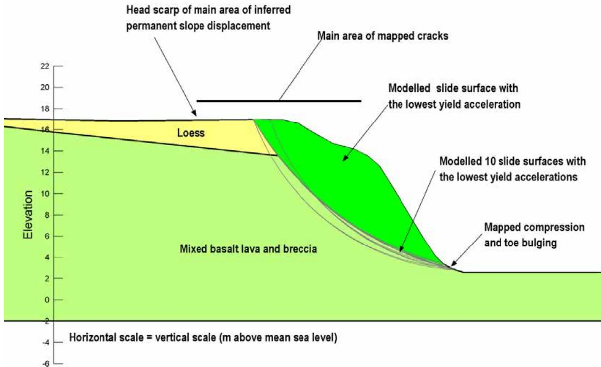
**Figure 22** Source area 11B (cross-section 1) seismic slope stability assessment for the 22 February 2011 earthquake. Failure mechanism 2, relatively shallow failure through the rock. The slide surface, and associated slide mass, with the lowest yield acceleration is shown bright green in colour.
