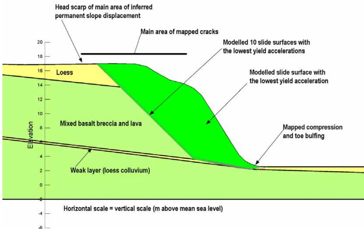
**Figure 23** Source area 11B (cross-section 1) seismic slope stability assessment for the 22 February 2011 earthquake. Failure mechanism 3, failure of rock through the weak layer within the rock mass. The slide surface, and associated slide mass, with the lowest yield acceleration is shown bright green in colour.
