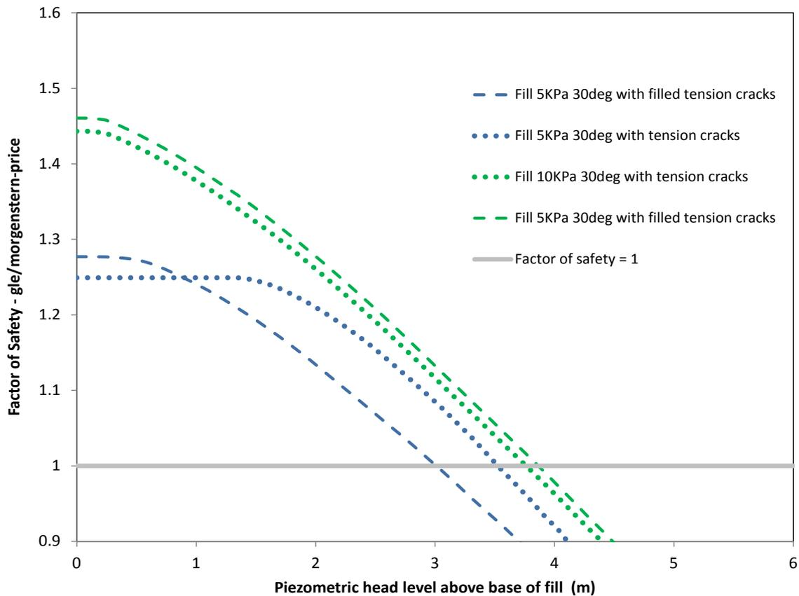
**Figure 11** Sensitivity assessment of the slope factor of safety (source area 11A) in response to changing piezometric head levels and tension crack conditions. Variable tension crack depths have been used.
