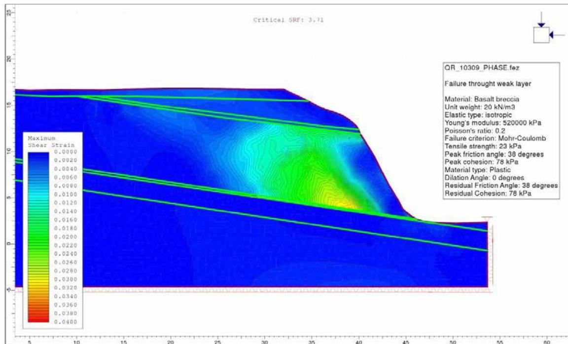
**Figure 16** Example of limit equilibrium and finite element modelling results for cross-section 1, representing source area 11B, for failure mechanism 3 through the weak layer.
