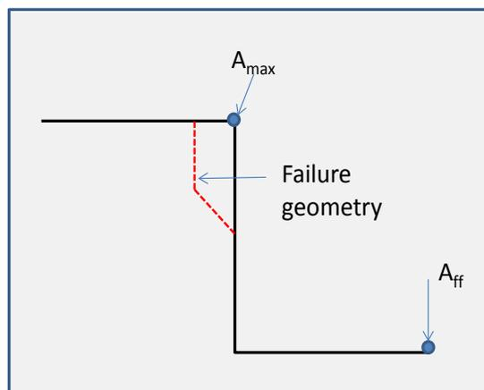
**Figure A3.1** Amplification relationship between the synthetic free-field rock outcrop input motions ( $A_{FF}$ ) and the modelled cliff crest maximum accelerations ( $A_{MAX}$ ) for cross-sections 1 and 2. A schematic diagram showing the locations of the various recorded accelerations is shown.
