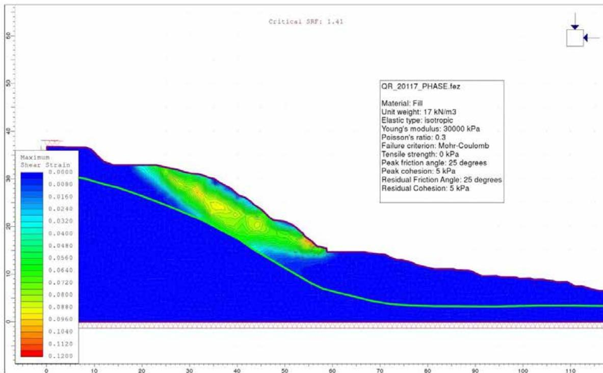
**Figure 13** Example of limit equilibrium and finite element modelling results for cross-section 2, representing source area 11A.
