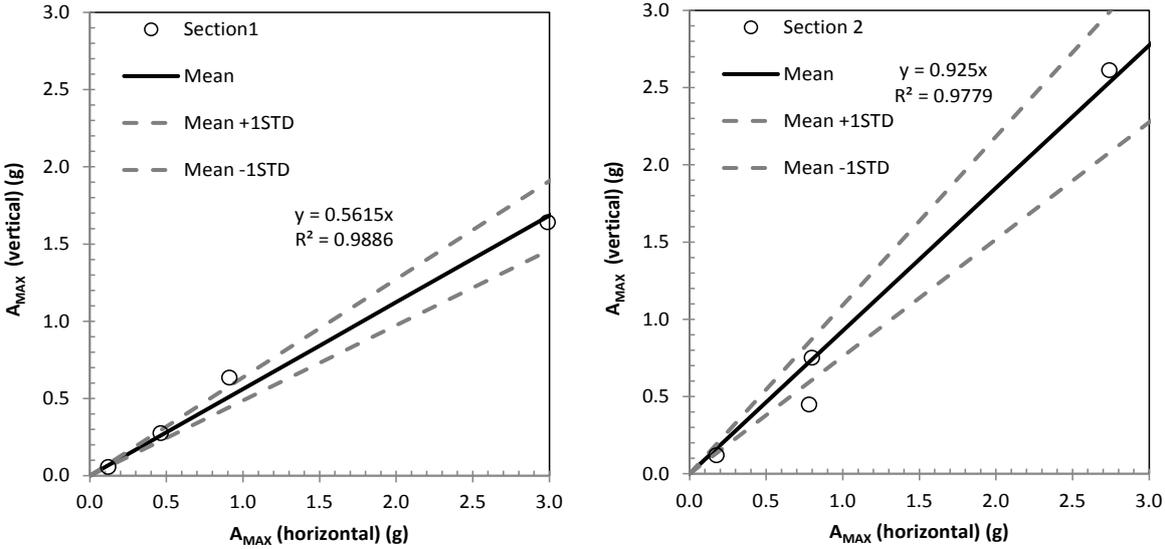
**Figure A3.3** Relationship between the modelled horizontal and vertical maximum accelerations modelled at the slope crest ( $A_{MAX}$ ) for cross-sections 1 and 2, using the synthetic free-field rock outcrop motions for the Quarry Road site by Holden et al. (2014) as inputs to the assessment. The mean and standard deviation trend lines are fitted for  $A_{MAX}$  all data. Errors are shown as the mean  $\pm$  one standard deviation (1 STD).
