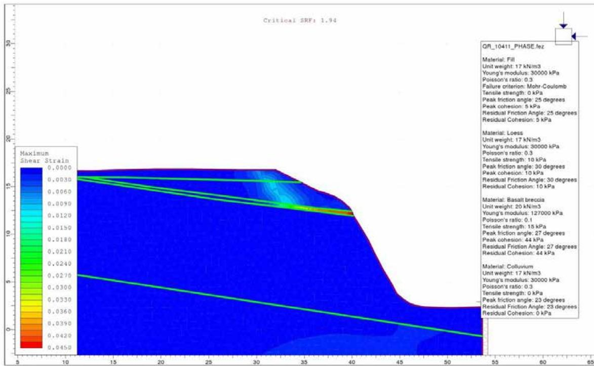
**Figure 14** Example of limit equilibrium and finite element modelling results for cross-section 1, representing source area 11B, for failure mechanism 1 through the loess.
