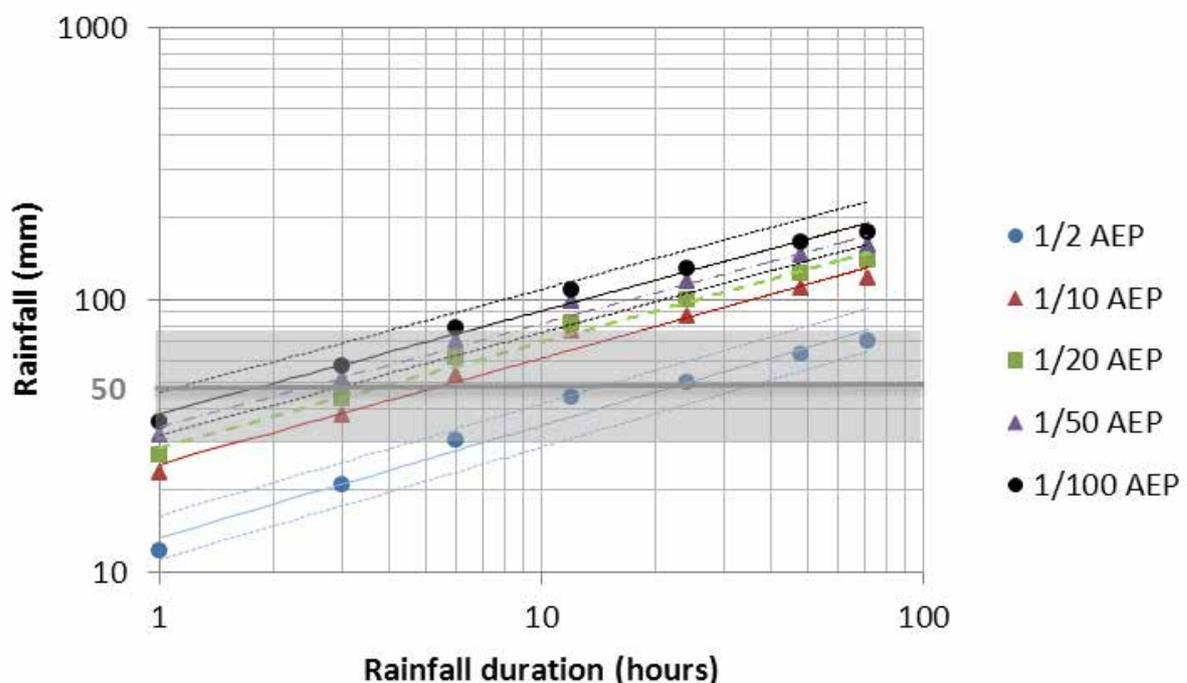
**Figure 10** Rainfall depth-duration-return period relations estimated by Griffiths et al. (2009) using recorded rainfall data. Error limits of 20% are shown by dotted lines for the 1/2 and 1/100 AEP curves. Shaded area covers the range of 30–75 mm of rainfall over which the expected number of soil landslides in the Port Hills rises from very few to many. Rockfalls can occur without rain, but the probability of rockfalls occurring increases with increasing intensity of rainfall.
