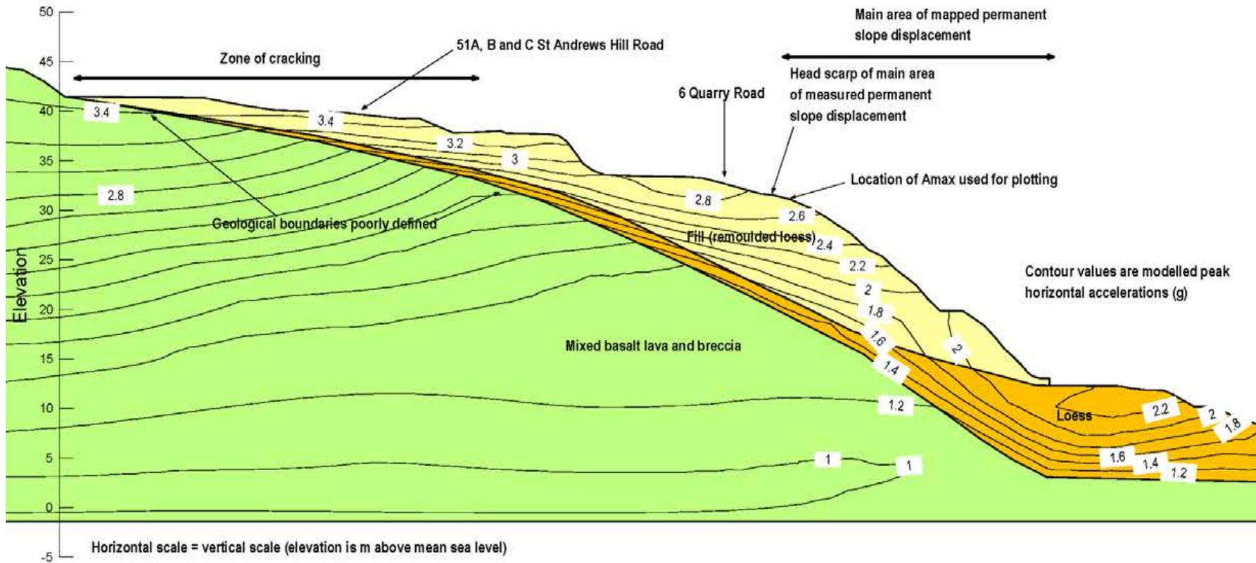
**Figure A3.2** Modelled peak horizontal ground acceleration contours for the 22 February 2011 earthquake at Quarry Road, source area 11A (cross-section 2). Note: the high peak horizontal ground accelerations shown at the left of the drawing are not thought realistic as the geological boundary conditions in this area are unknown and have been inferred.
