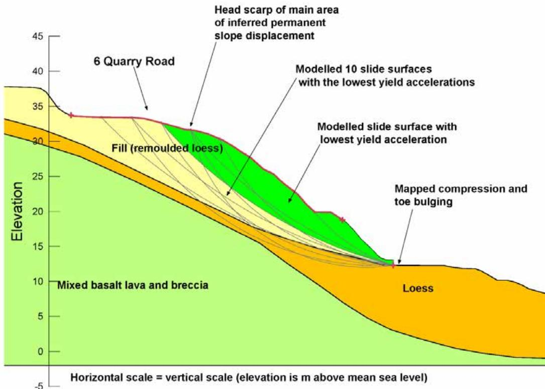
**Figure 20** Source area 11A (cross-section 2) seismic slope stability assessment for the 22 February 2011 earthquake. The slide surface, and associated slide mass, with the lowest yield acceleration is shown bright green in colour.
