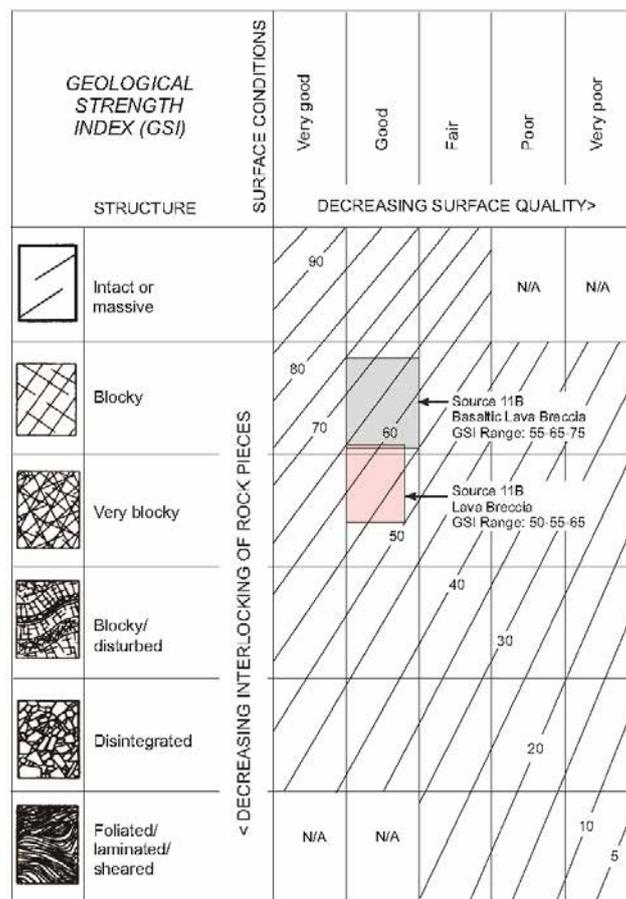
**Figure 8** Geological strength index plot for volcanic breccia at Quarry Road (modified after Hoek, 1999).
