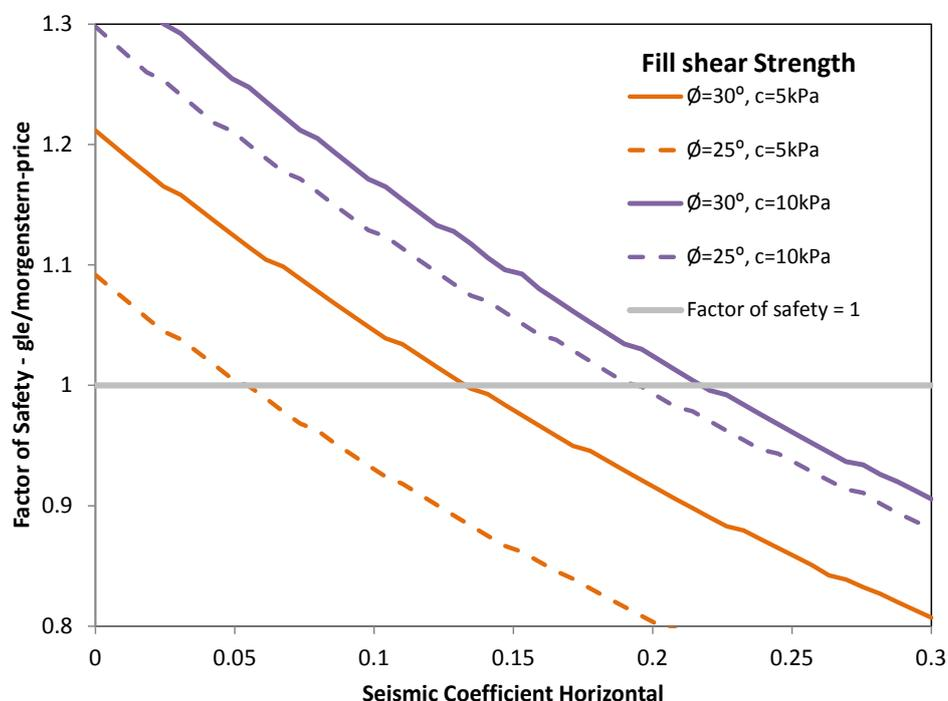
**Figure 26** Yield acceleration of the slope based on variable fill parameters and loess parameters shown in Table 11. Yield acceleration calculated adopting the pseudostatic method (Kramer, 1996).
