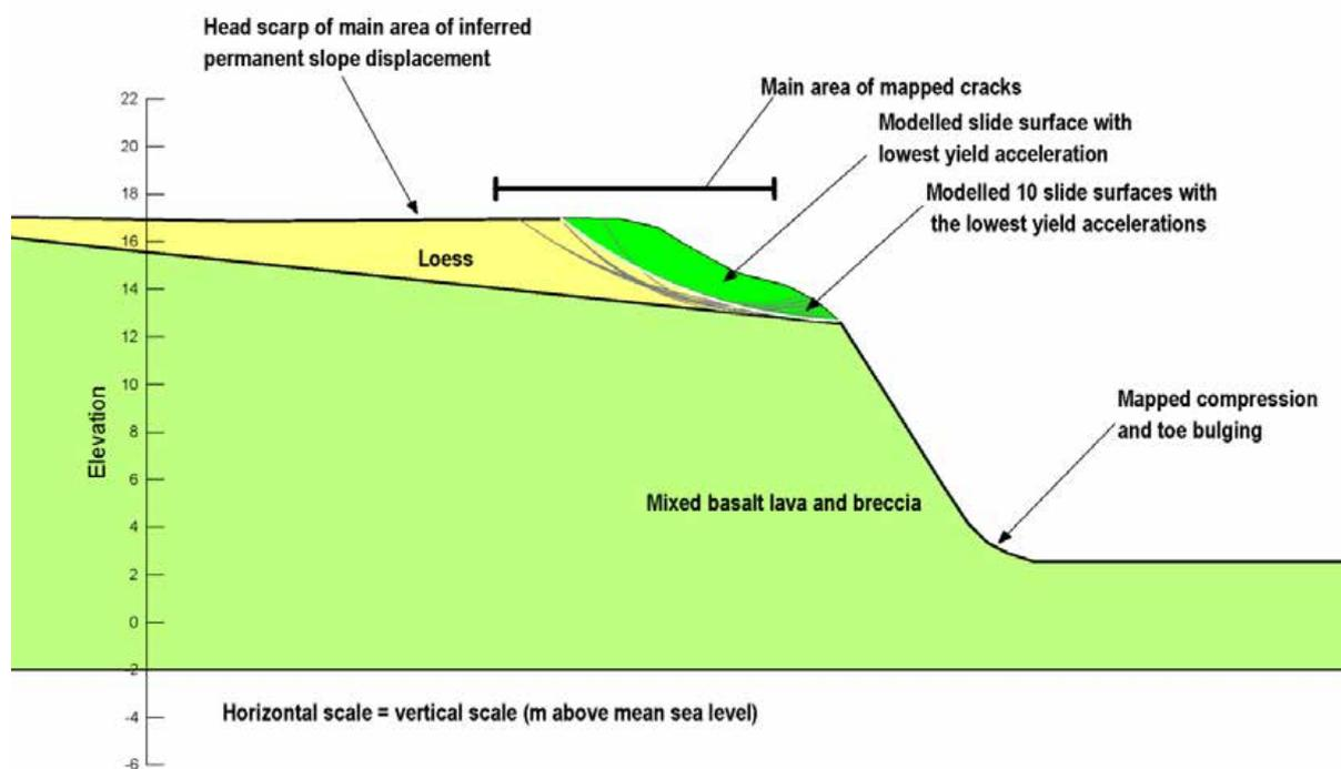
**Figure 21** Source area 11B (cross-section 1) seismic slope stability assessment for the 22 February 2011 earthquake. Failure mechanism 1, failure through the loess only. The slide surface, and associated slide mass, with the lowest yield acceleration is shown bright green in colour.
