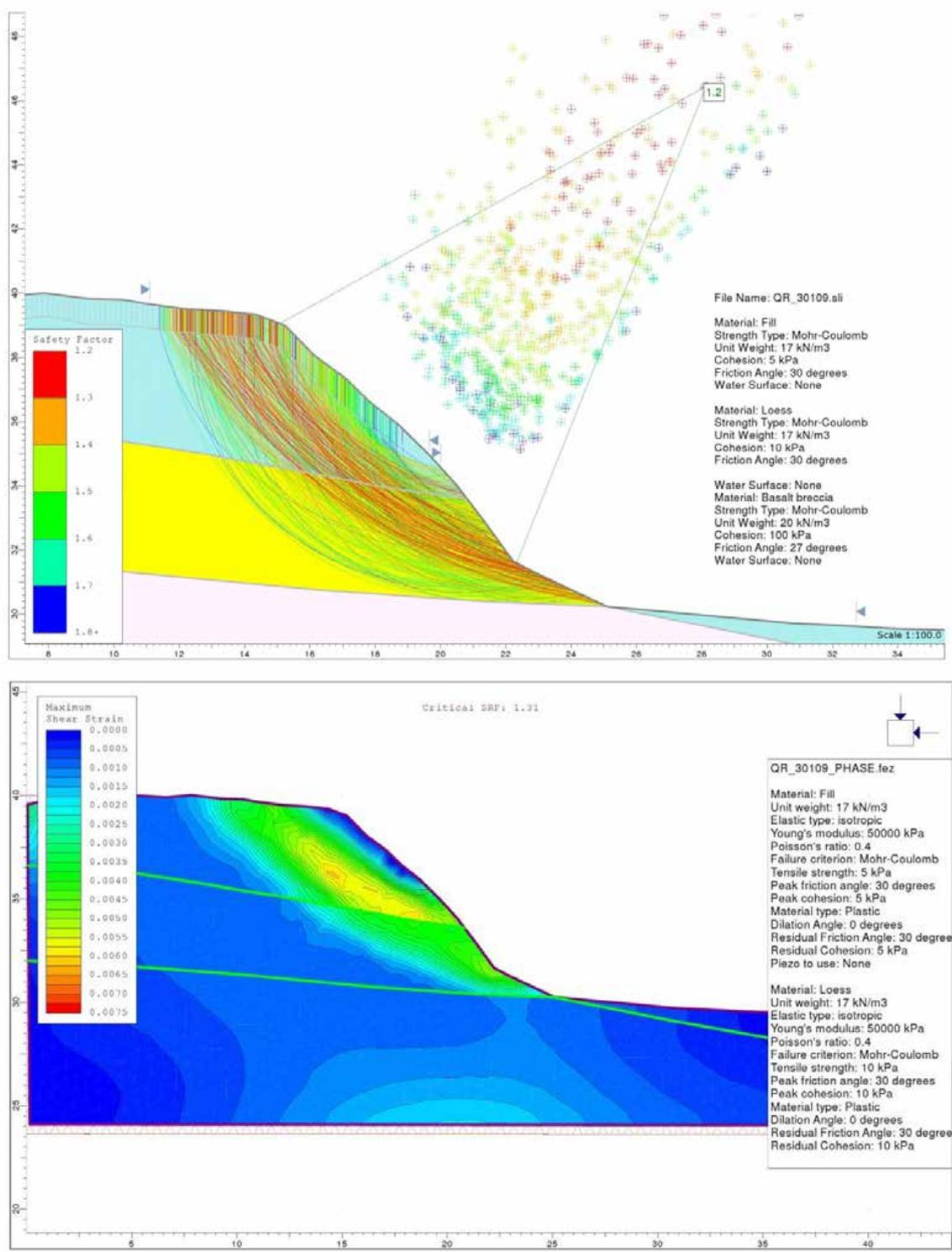
**Figure 17** Example of limit equilibrium and finite element modelling results for cross-section 3, representing source area 11C, for a failure mechanism through the fill and loess.
