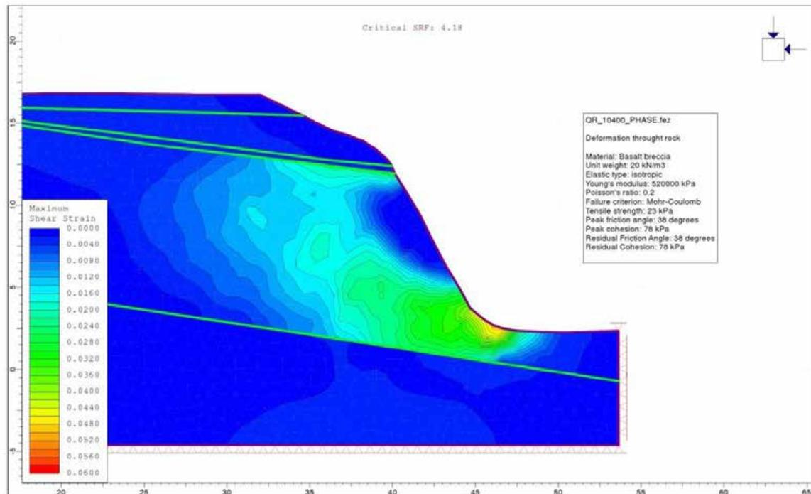
**Figure 15** Example of limit equilibrium and finite element modelling results for cross-section 1, representing source area 11B, for failure mechanism 2 through the rock.
