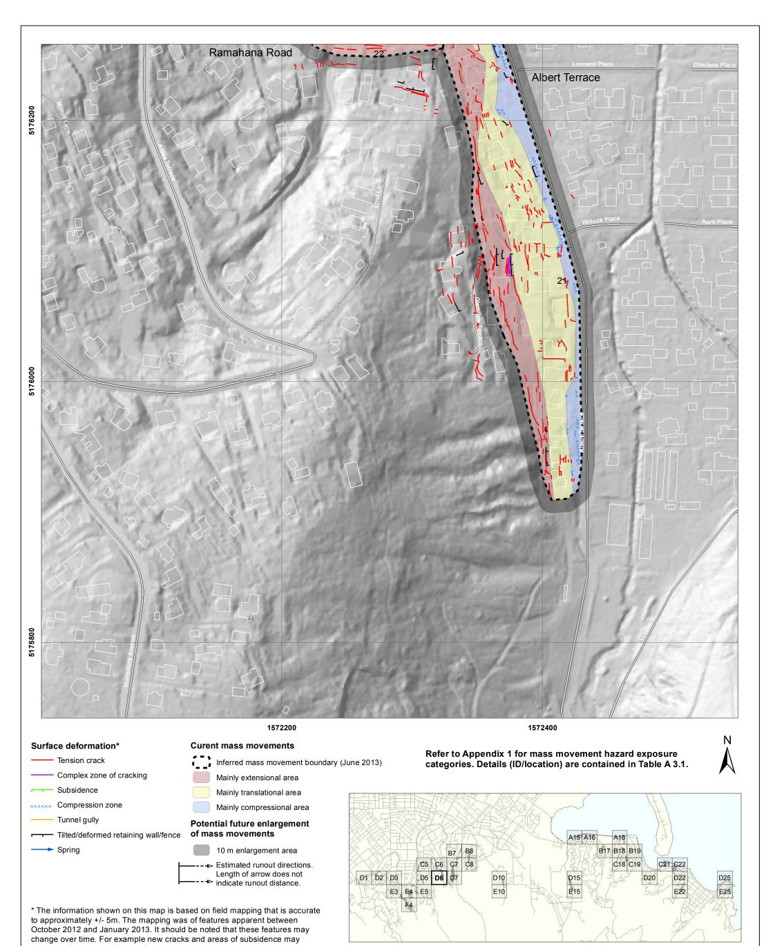
appear and some cracks may disappear. SCALE BAR: 50 100 ⊐ m **STAGE 1: MASS MOVEMENTS** DRW: **EXPLANATION:** Background shade model derived from NZAM post earthquake 2011c (July 2011) LiDAR survey resampled to a 1 m ground resolution. CHK: CM Roads and building footprints and types provided by Christchurch **Port Hills** JC, MY City Council (20/02/2012). Christchurch PROJECTION: New Zealand Transverse Mercator 2000
