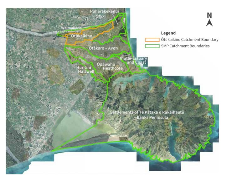
The boundaries of the seven stormwater management catchments within the area covered by the Comprehensive Stormwater Network Discharge Consent.
