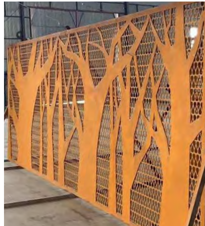
1. Decorative laser cut steel panel fence and gates
