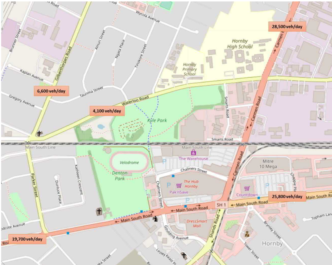
Figure 2-2: Traffic Volumes on Surrounding Roads
