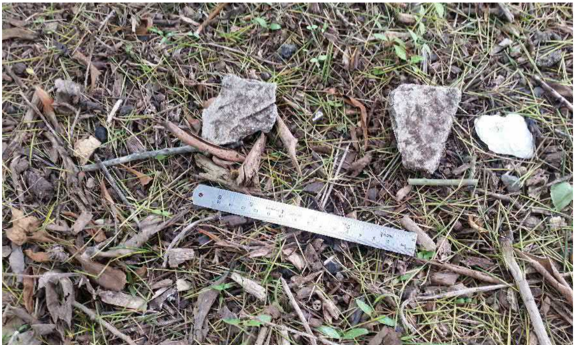
Above: Photograph 10 - example of ACM fragment, in-situ (Area 2)
