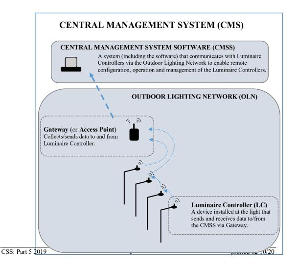
The Outdoor Lighting Network is an Itron Network Solutions mesh network.
