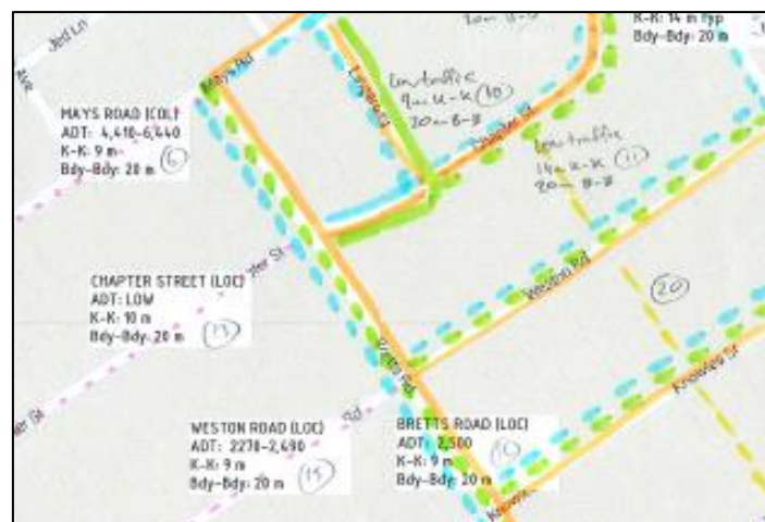
Figure 6-2: Individual Road / Path details
