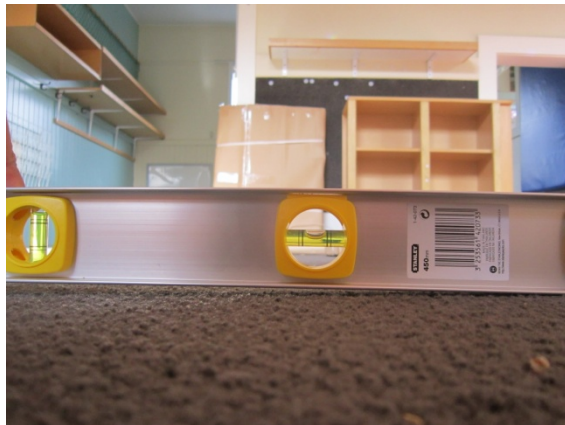
Photo 31: Estimating the slop using a spirit level
