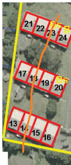
Figure 8: Locations of ground crack through blocks D, E and F.
