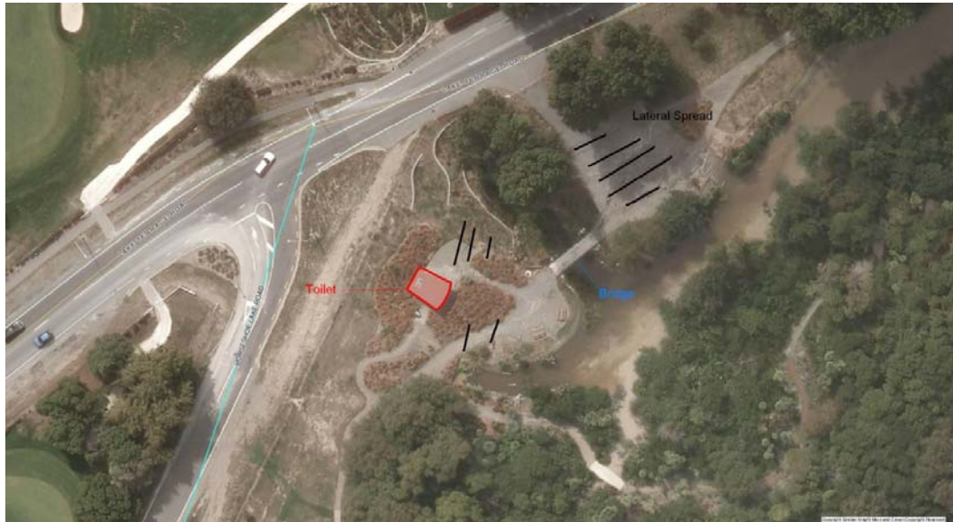
■ Figure 8 Overview map showing alignment and distribution of tension cracks
