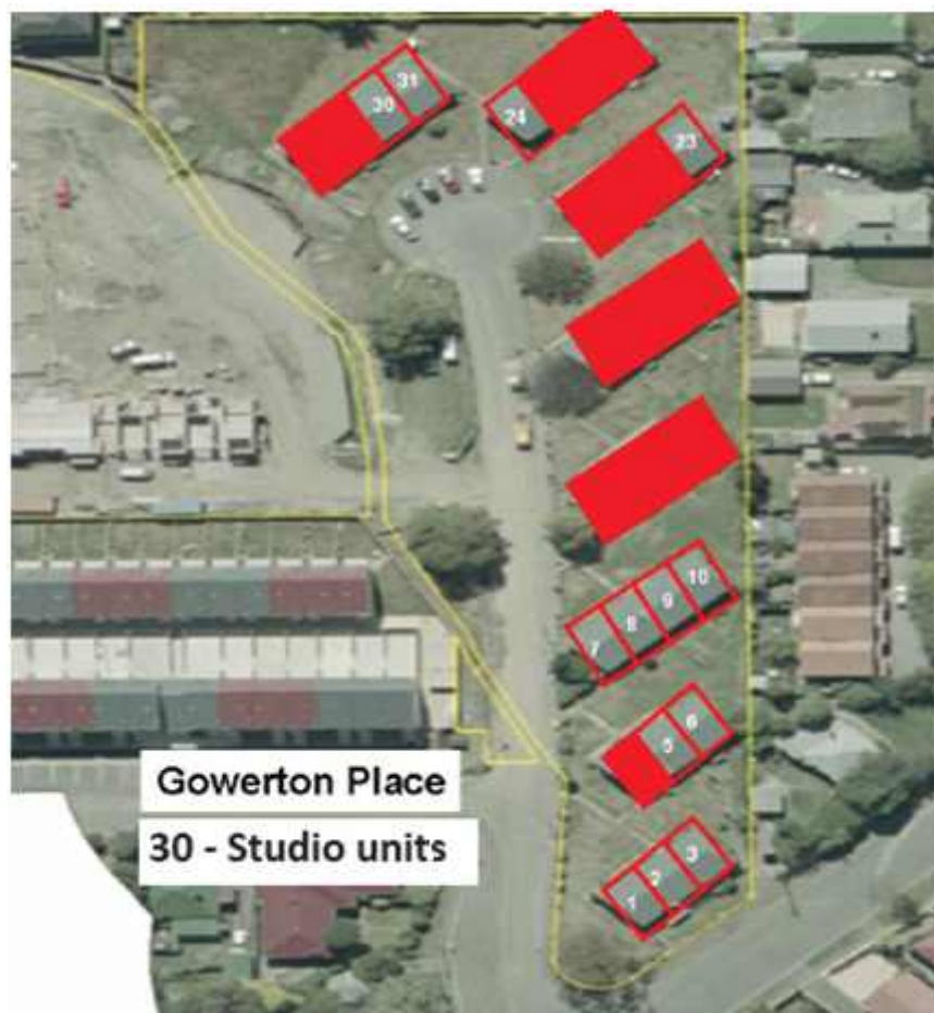
Figure 6: Units which have floor slopes exceeding 5mm/m (coloured red).
