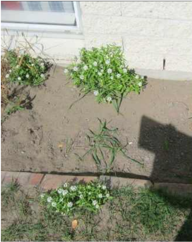
Photograph 15: View of possible ejected liquefied material observed in the flower beds surrounding the residential units.
