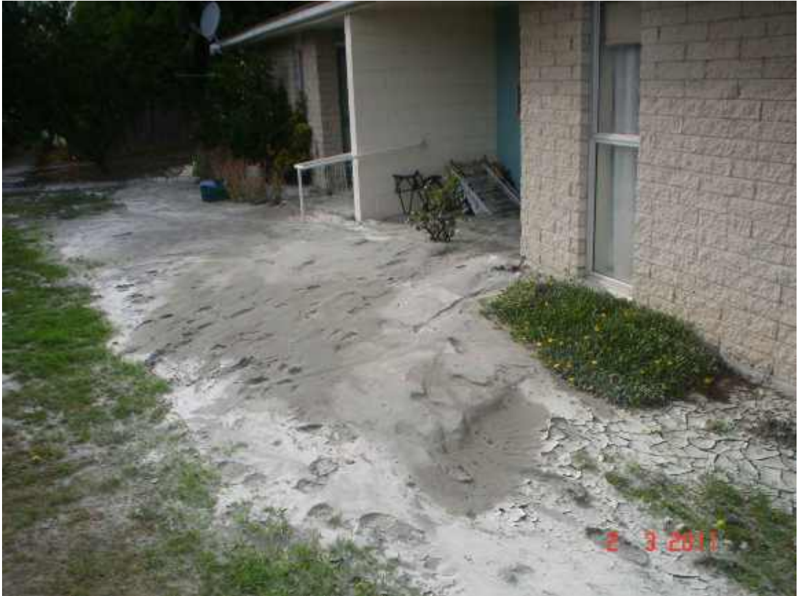
Photograph 17: View of ejected liquefied material (Photograph taken in March 2011).
