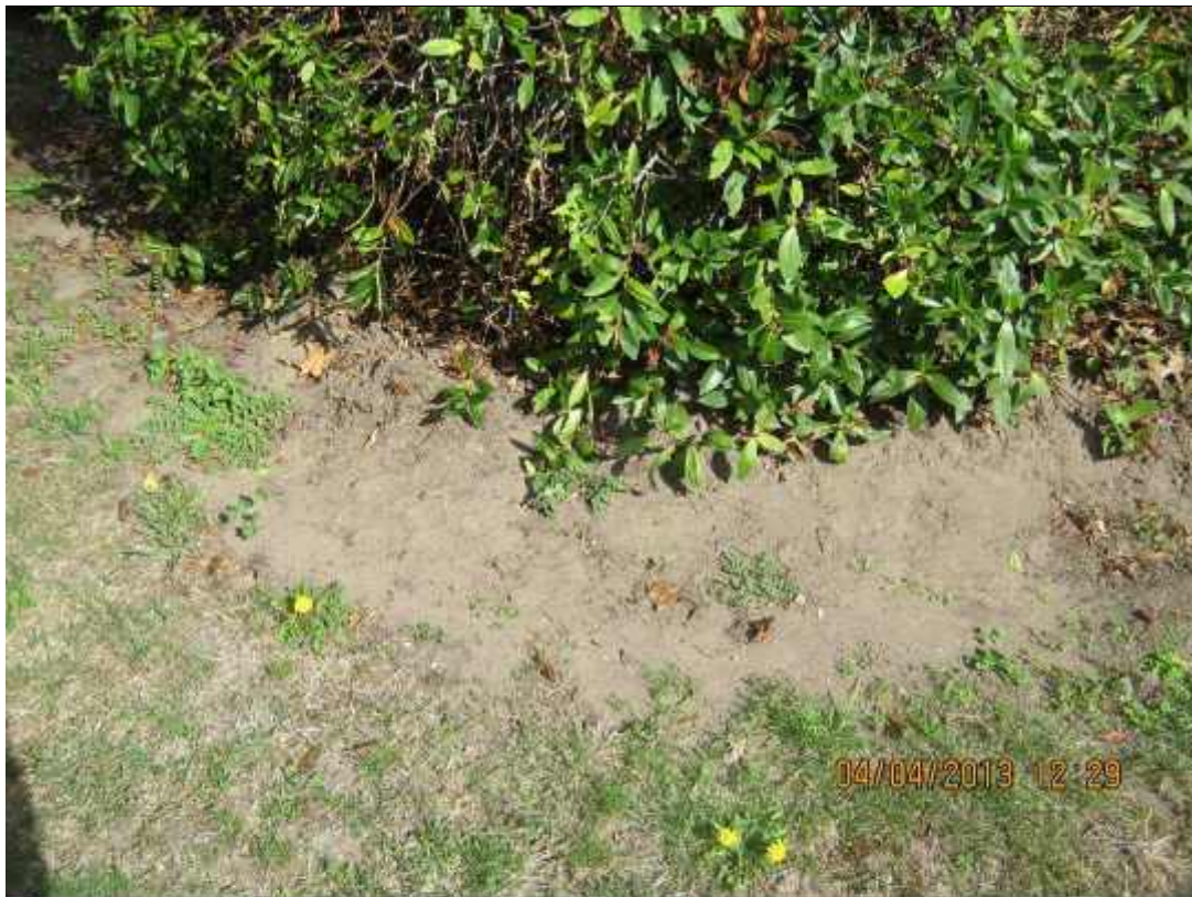
Photograph 11: View of sand boil observed in southwestern corner of site.
