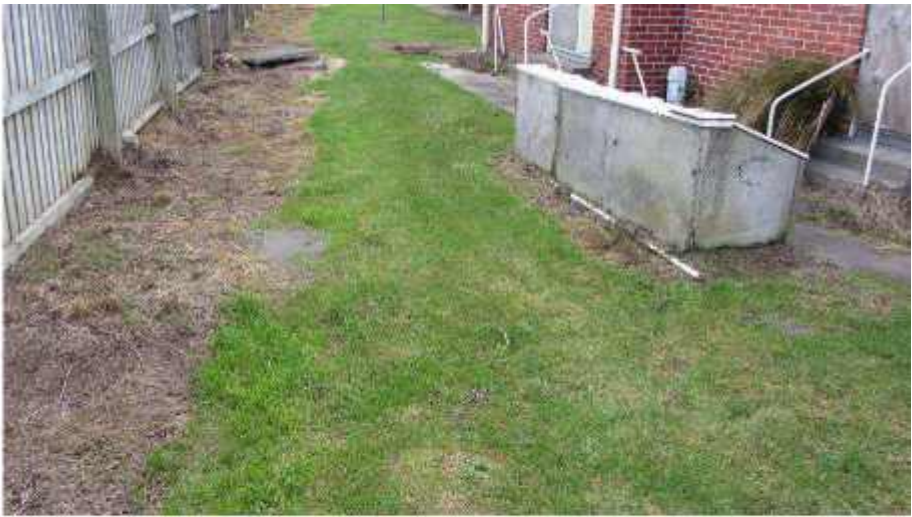
Photo 46: SILT/SAND Ejecta behind Flat 21 Looking Southwest
