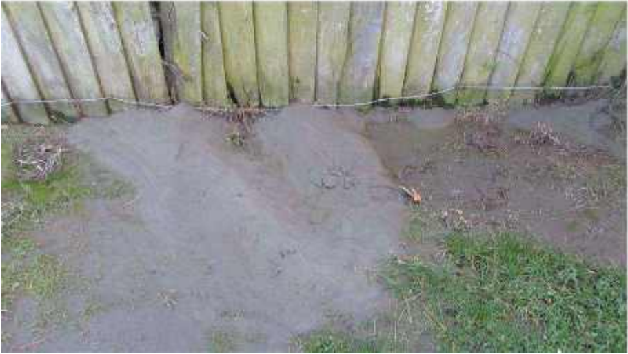
Photo 47: SILT/SAND Ejecta behind Flat 26 Looking Northwest
