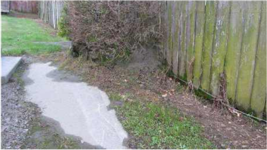
Photo 48: SILT/SAND Ejecta behind Flat 26 Looking West
