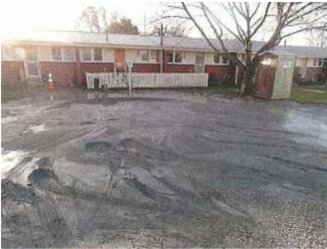
Photo 9: View Liquefaction at Cresselly Place and Even-Numbered Flats 20-26 Looking North-Northeast; Photo taken 14 June 2011
