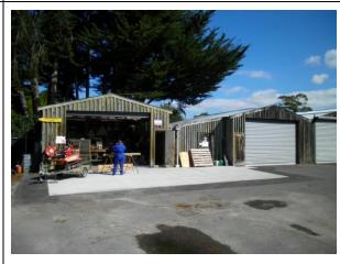
New additions evidenced by building paper and lighter colouration on the timber
