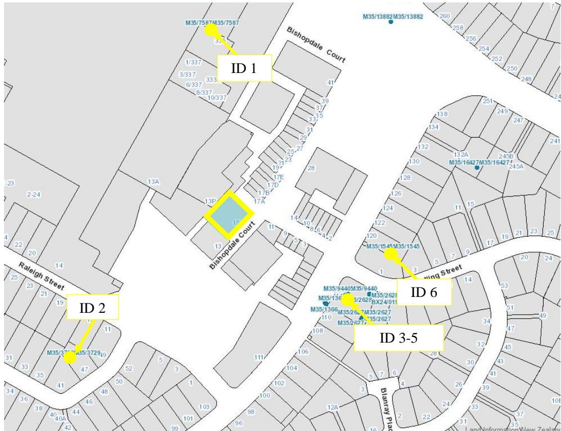
■ Figure 6 – Location of local ground investigations from ECan GIS ( http://canterburymaps.govt.nz/Viewer/ )
