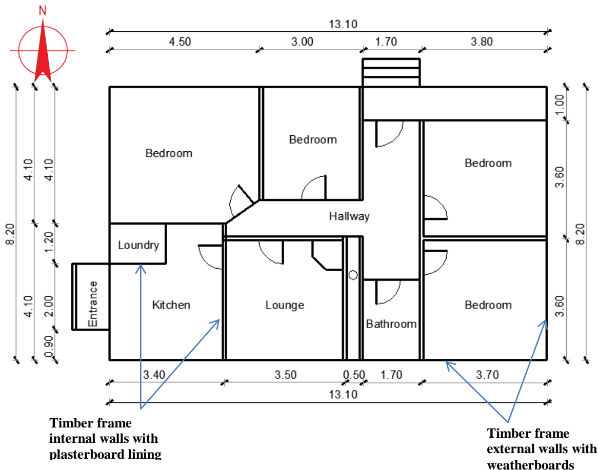
Figure 2 Plan Sketch Showing Key Structural Elements
