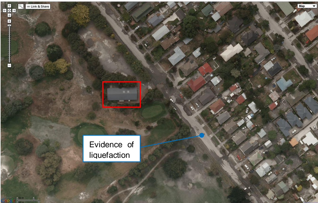
Photo 2: Liquefaction of areas surrounding site (aerial photo taken 24 February 2011)
