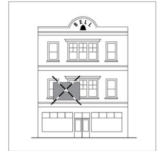
Building identification sign. Conflict with architectural features
