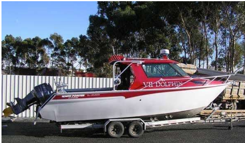
Photograph 1 – An example of a vessel similar to the design power boat (8.2m LOA, 2.5m beam)
