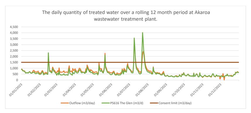
The volume of treated wastewater discharged can exceed the consent limit of 1,500 cubic metres per day during rainfall events of a total of 50 millimetres or more over three consecutive days.
