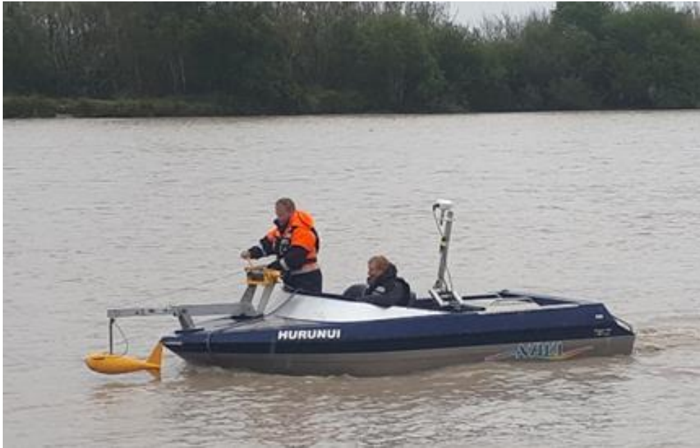
Figure 2-2: P-61 suspended sediment sampler deployed from jetboat on Waimakariri River.
