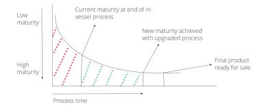
The current system processes material for about 14 days in the composting vessels to the maturity noted on the graph, this is the active composting phase. The remainder of the composting process (maturing and curing) happens outside in windrows over about 12 weeks.
