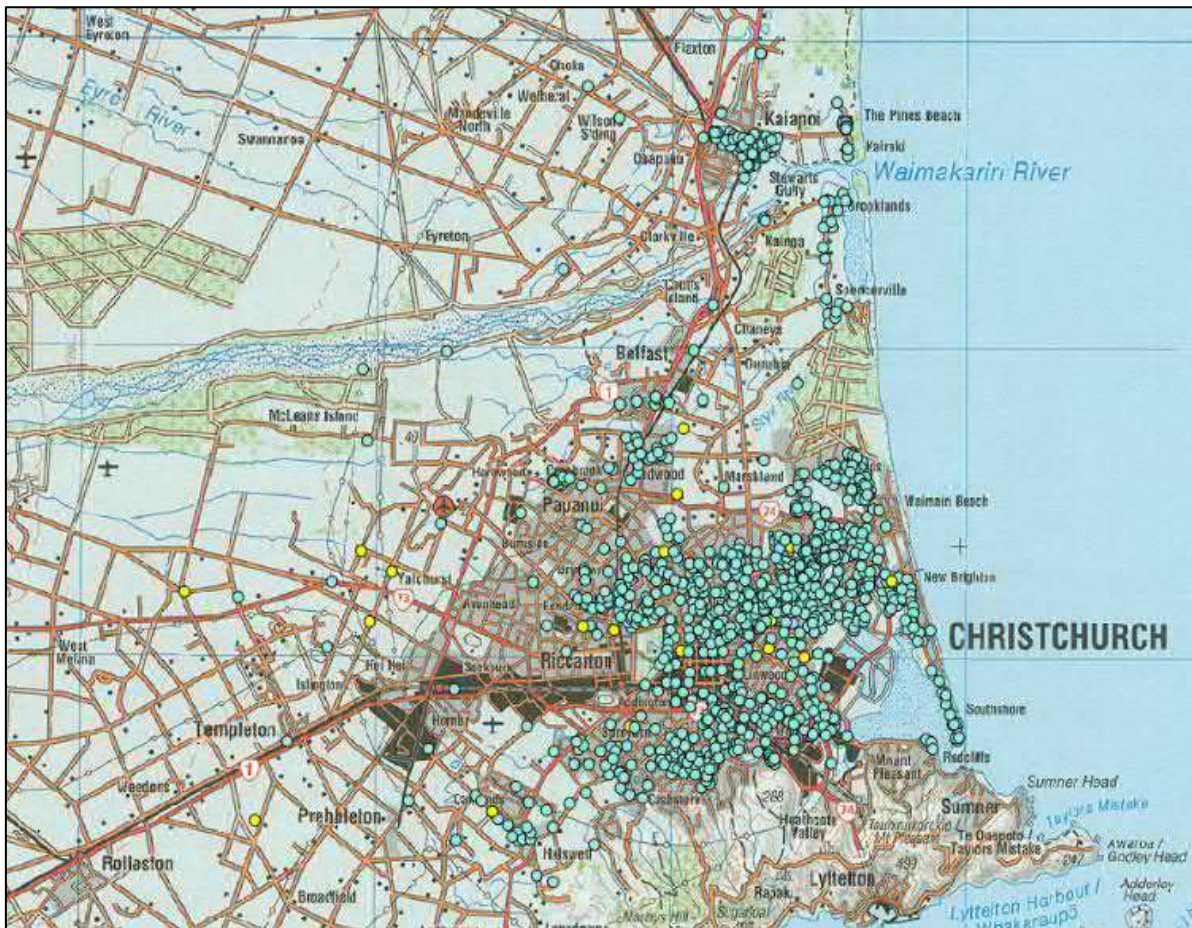
Figure 37. Groundwater depth observation sites. Yellow dots are those sites with the greatest shift in medians before and after November 2013
