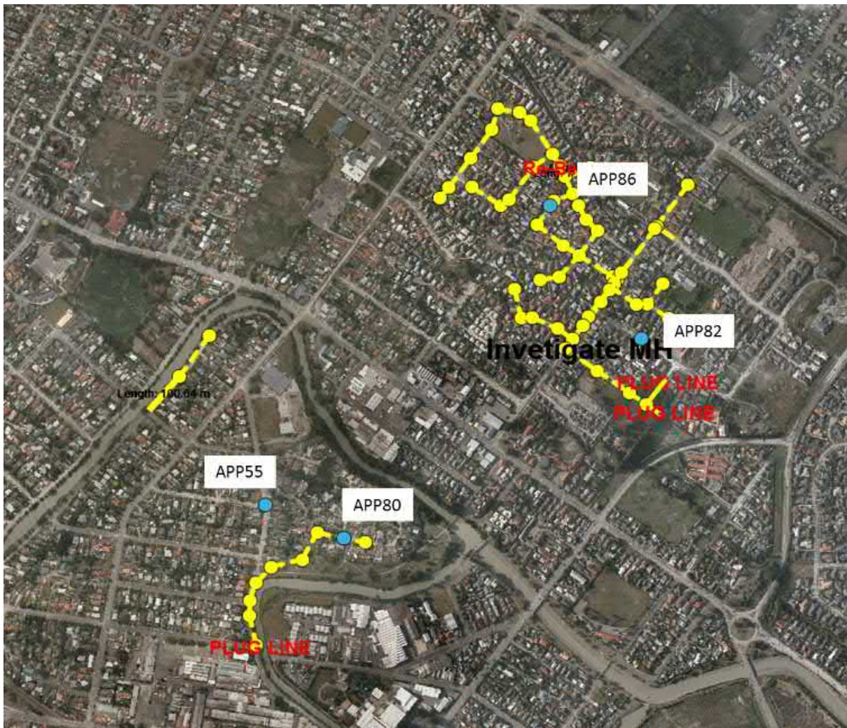
Figure G.1: Location of APP piezometers in the Woolston area, and sewer lines that are due to, or have been, decommissioned.
