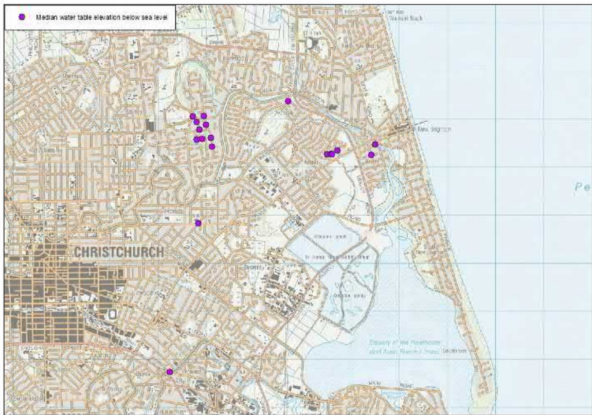
Figure 39. Piezometers with median groundwater elevation below sea level
