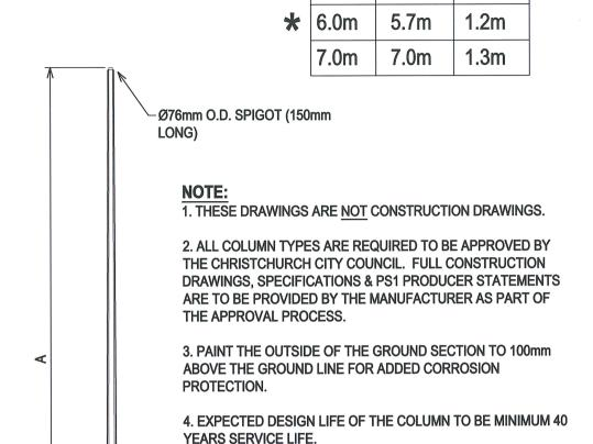
5. THIS COLUMN CAN BE USED AS A PEDESTRIAN CROSSING COLUMN. WHEN USED IN THIS SITUATION COLUMN IS TO BE PAINTED GLOSS BLACK (RAL 9004) AND HAVE 300mm WIDE WHITE PAINTED PARALLED STRIPS ALTERNATE TO 3m ABOVE
